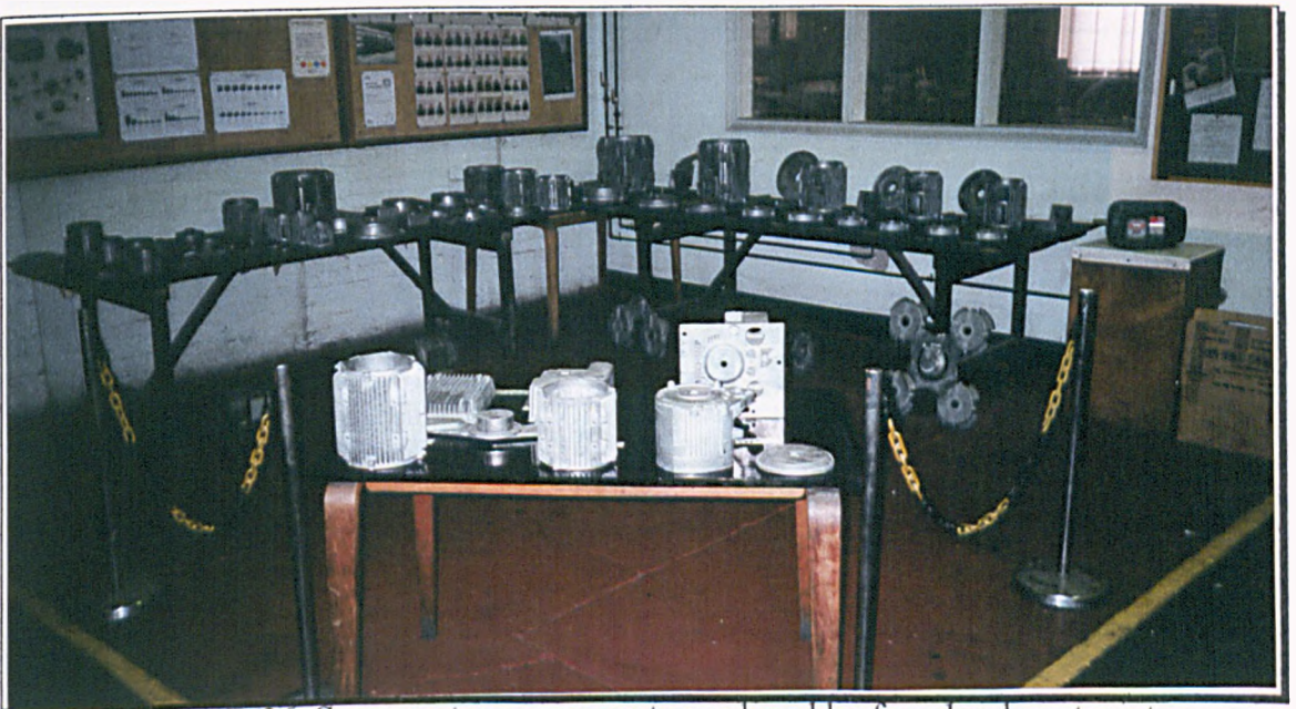
Figure D.36. Some motor components produced by foundry department.
