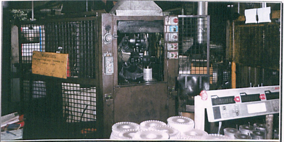
Figure D.18. The automated rotor production station.
