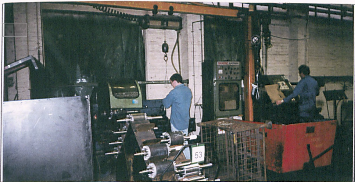
Figure D.27. Machining operation for sub-assemblies of rotors.
