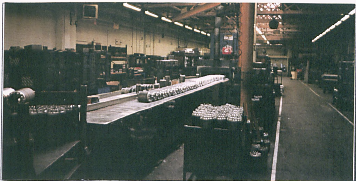
Figure D.26. The first part of rotor assembly line.
