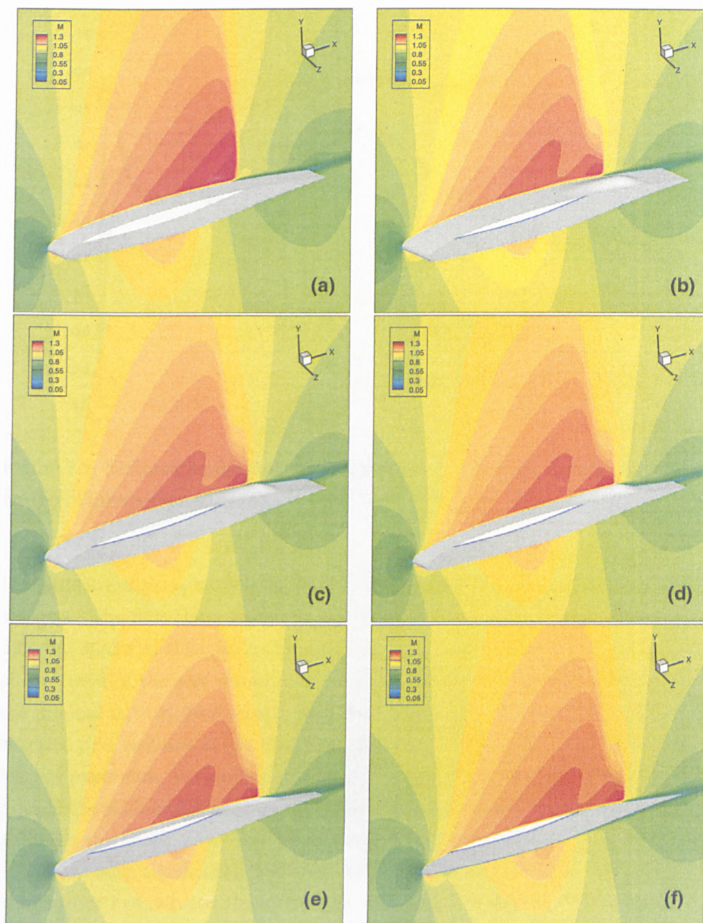
Figure 7.7: (a) Mach number contours of the original normal shock wave. (b) Mach number contours along the tip of the optimised 3D bump. (c) Mach number contours along the mid-span of the optimised 3D bump. (d) Mach number contours along the centreline of the optimised 3D bump. (e) Mach number contours along the mid-span of the optimised 3D bump. (f) Mach number contours along the tip of the optimised 3D bump. (On the infinite swept wing, M_\infty = 0.85 , C_L = 0.32 .)
