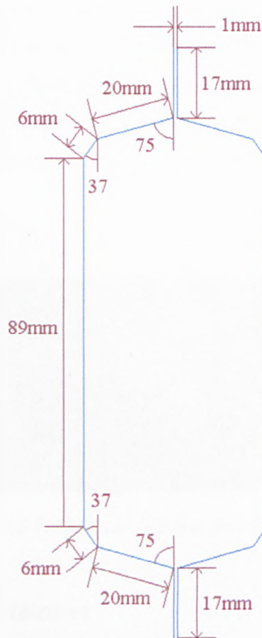
Figure 12.6: Final design for the spot-welded component
