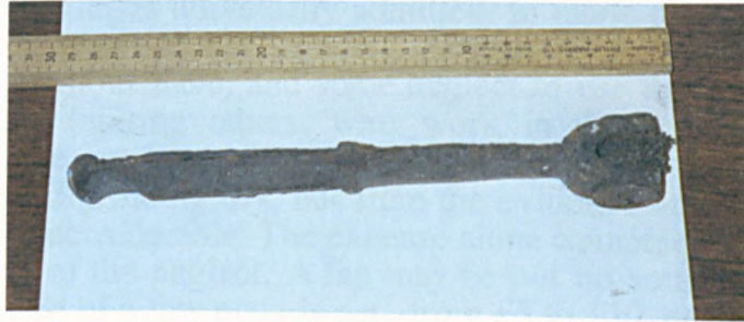
Figure 19: Racing iron, used to true up irregularities on a grindstone. Found at Butcher's Wheel (Sept 1995)
