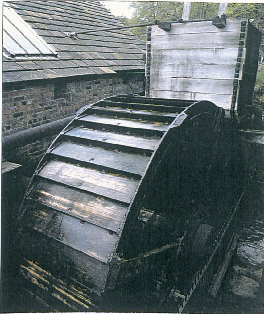
Figure 17: Wheels at Abbeydale. A: Tilt Hammer Wheel and B: Wheel for driving grinding stones and blowing engine. (From Abbeydale Industrial Hamlet, Sheffield City Museums 1981 pp13-14)
