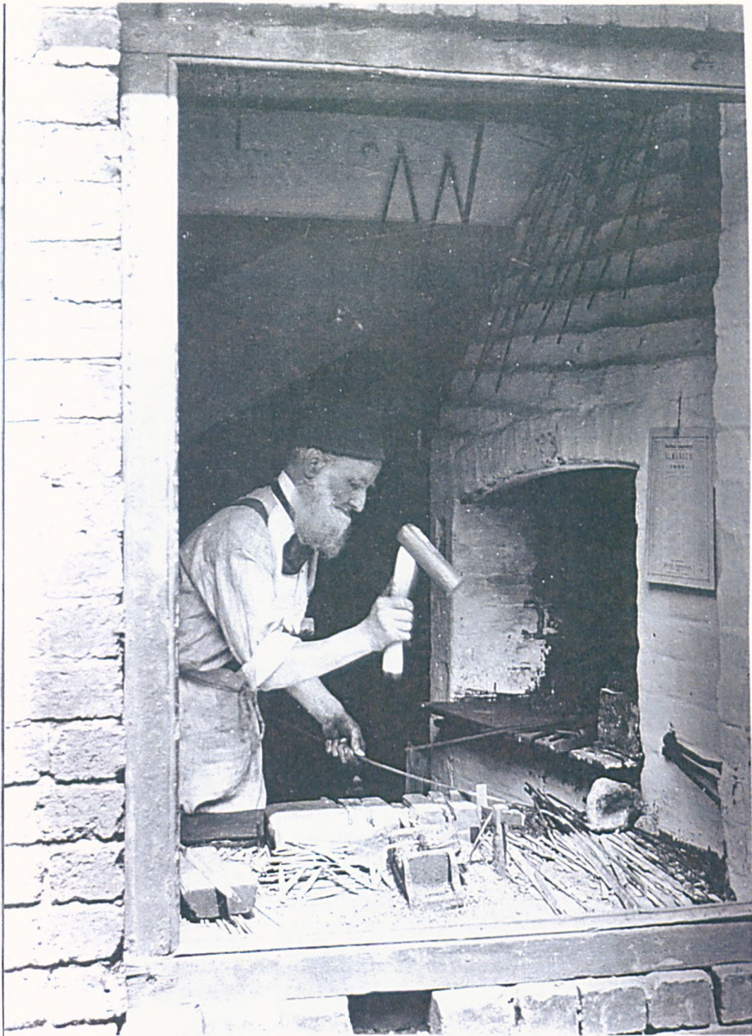
Figure 4:File Forging, Thomas Turner's 1902. Note the agon (A1) and the difference in the shape of the anvil when compared to the blade forger's anvil (figure 3). Note the stepped breast of the forger's hearth and the shape of the hammer and the handle of the hammer worn after years of use thus marking clearly where the hammer was held. ( Handicrafts that Survive p55 )
