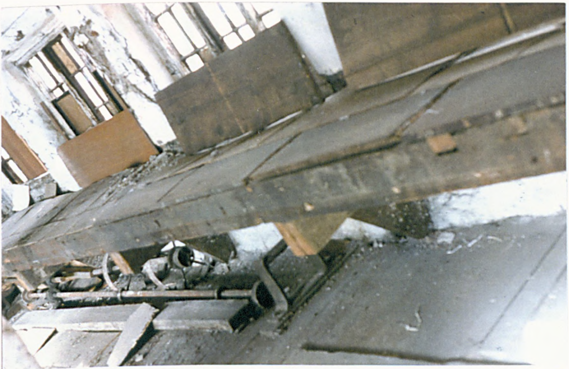
Figure 22b: Workbench at Kendal Works, made up of short lengths of timber. Note line shaft under bench. (Photo: Sanella, 1994)
