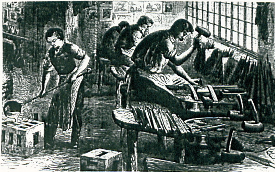
Figure 27: London Illustrated News 1866, File cutting. Note the lead bed being teemed in front of the fire place (A1). The characteristic file cutters windows and hammers can also be seen.
