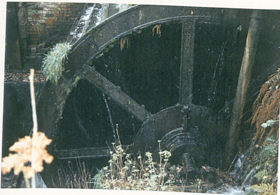
Figure 18: The iron wheel which survives at Low Matlock (Loxley), although it has now been set back off its bearings.
