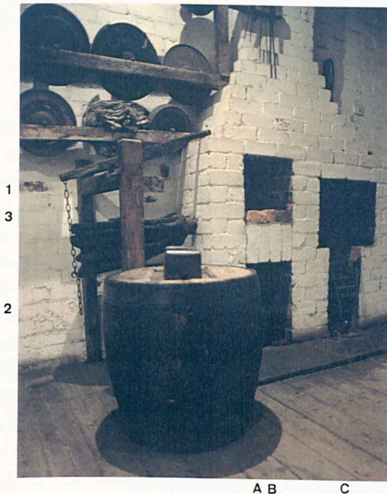
Figure 9: Cutler's Hearth, Kelham Island. Note the three openings for hardening (A1), the ash hole (B2) and the fireplace (C3). The 'long shaped bellows' are mounted on a wooden frame to which an extended handle is attached so that the cutler could observe the heat in the hearth and the metal.
