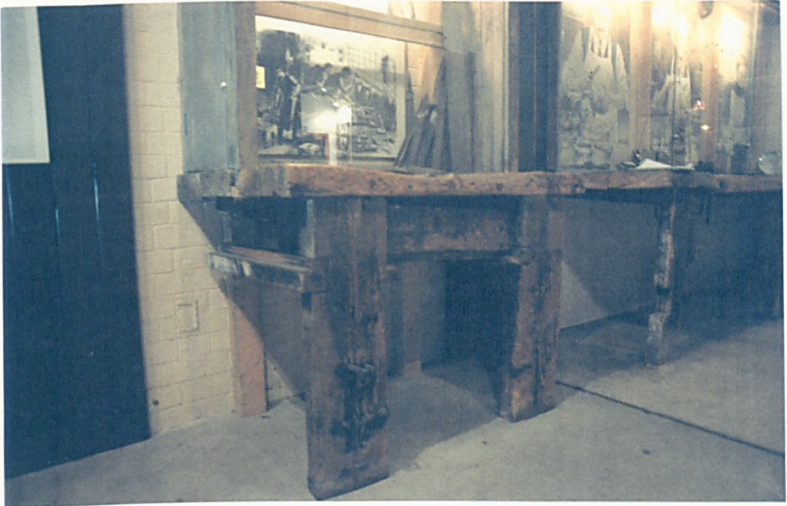
Figure 22a: Cutler's Workbench, Kelham Island. Note the thickness of the timber.
