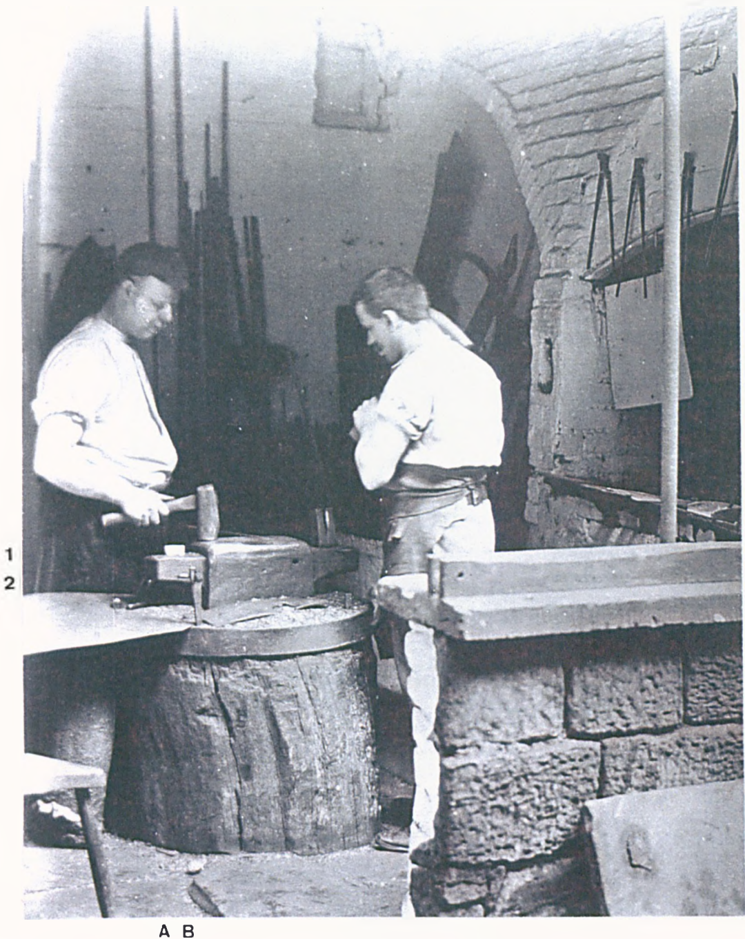
Figure 3: Double handed forging of Butcher's Blades at Thomas Turner's c1901. Note at A1 the 'agon' or upturned chisel used for cutting off the 'mood'. The spike at B2 is used to guide the forger when placing the blade over the agon. To the right of the photograph is the forger's hearth with its stepped chimney breast and the forger's tongs hang from it. The forgers hammers, weighing between four and twelve pounds have characteristically bent heads which made the swing more efficient. The same shape is also used for file cutters' hammers (see figure 28b). Note that the floor of the workshop is flagged. (Photograph from the Hawley Collection, University of Sheffield. Originally produced in Handicrafts that survive p20)
