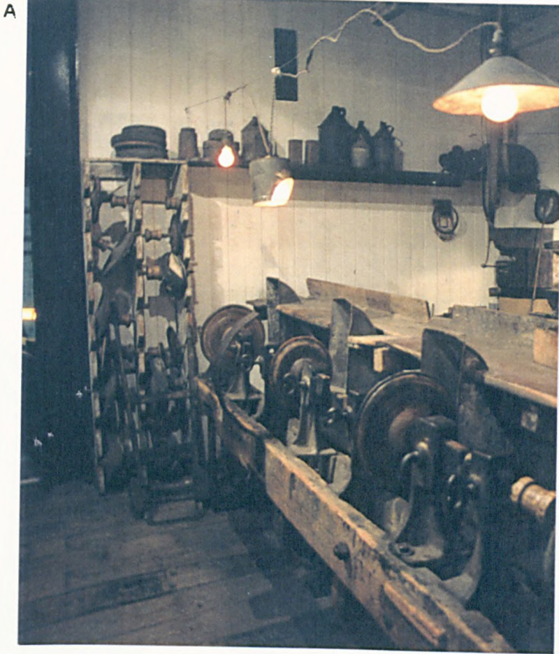
Figure 20 A : Extractor fans used with polishing machinery in display at Kelham Island set into the front of the bench and B : at A Wright and Son where they are set in the middle of the bench.
