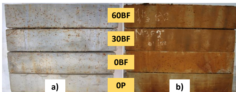
Figure 3.4: SFRRuC specimens after a) 150 days, and b) 300 days of wet-dry chloride exposure
