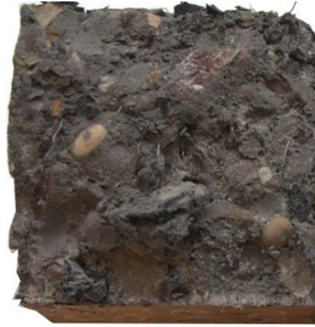
Figure 3.5: Section through a SFRRuC specimen after 300 days of wet-dry chloride exposure
