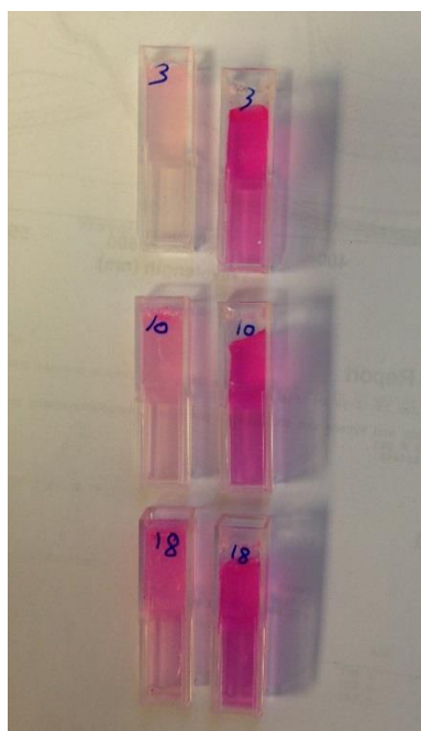
Figure 4-9: Decolourisation of MC 540 in SHG formulations in the presence of SDS at 3, 10 & 18 mM. The left-hand column contains 1.0 M formulation SHG and have been photographed after 3 h. The right-hand column has 0.5 M formulation SHG and is photographed after 28 h. The concentration of merocyanine is 0.01 mM in all cases.
