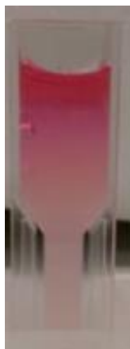
Figure 4-3: Photograph of a 1.0 M silica gel sample decolourising primarily from the bottom of the disposable cuvette to the top.
