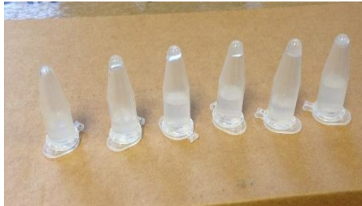
Figure 2-3: Identical samples of 0.5M SHG after 24 hrs in plastic tubes perforated earlier from the cap prepared in research lab for the CPD
