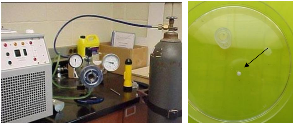
Figure 2-4: Critical point drying instrument within School of Biology, UoL (left). Dried SHG sample of 0.5 M concentration in a petri dish and the weight is 0.0156 g marked with black arrow (right).
