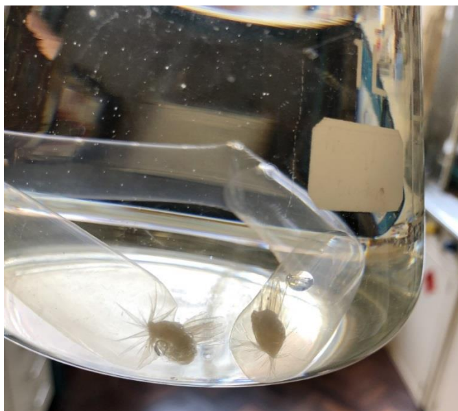
Figure 2-11: Dialysis tube contain SHG sample dissolved in water, tighten from ends and dipped in conical flask containing distilled water
