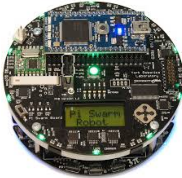
FIGURE 6.1: The Psi-Swarm robot used for the experiments in this chapter (Hilder et al., 2016).
