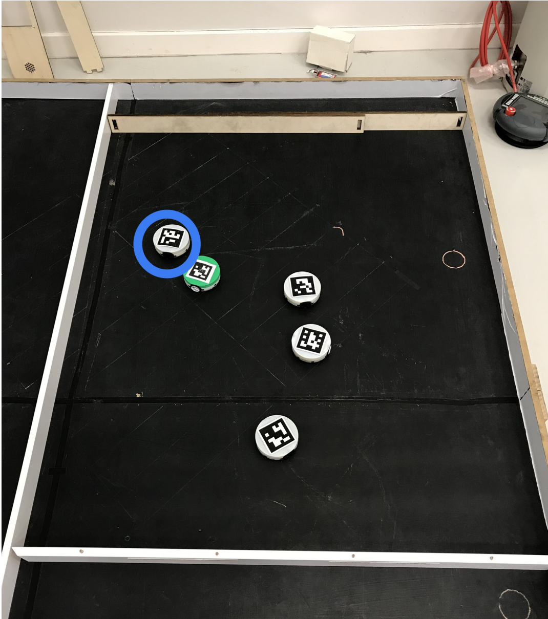
FIGURE 6.2: Five Psi-swarms performing obstacle avoidance in an arena. The robot with a green hat suffers from power failure ( H_1 ), whilst its assessing robot in this case is circled in blue.
