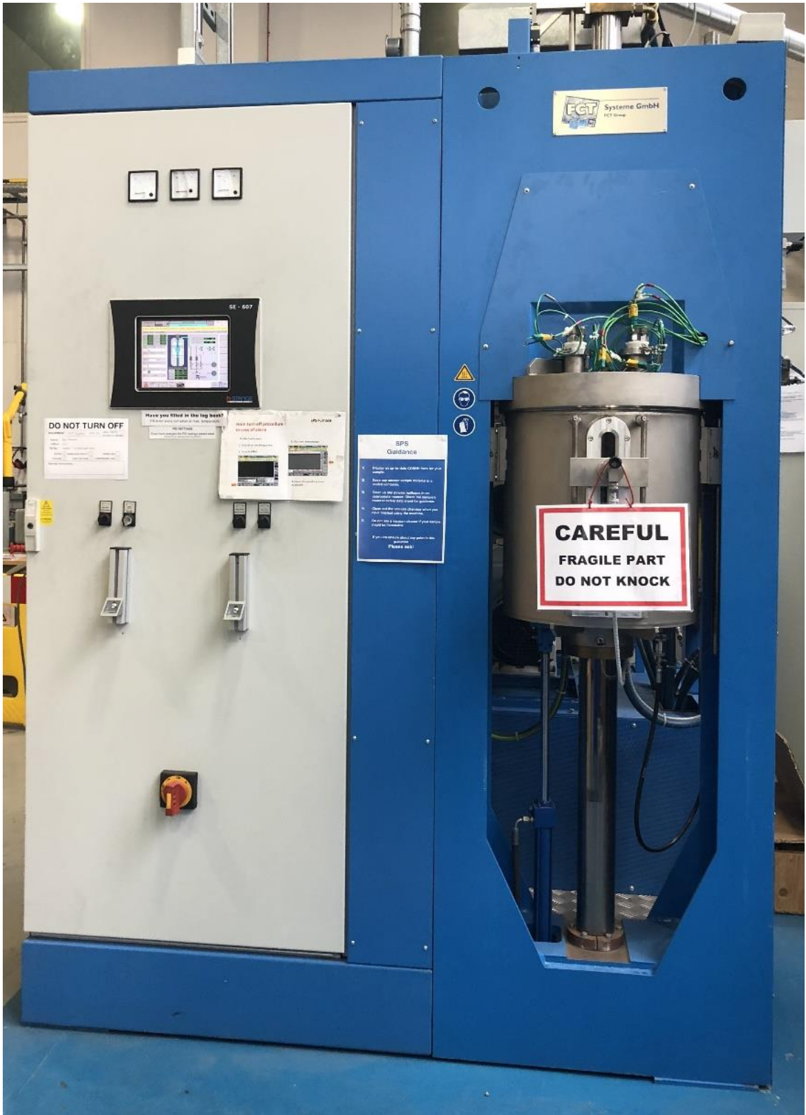
Figure 3.2 The FCT Systeme GmbH Spark Plasma Sintering furnace type HP D25 at the University of Sheffield.
