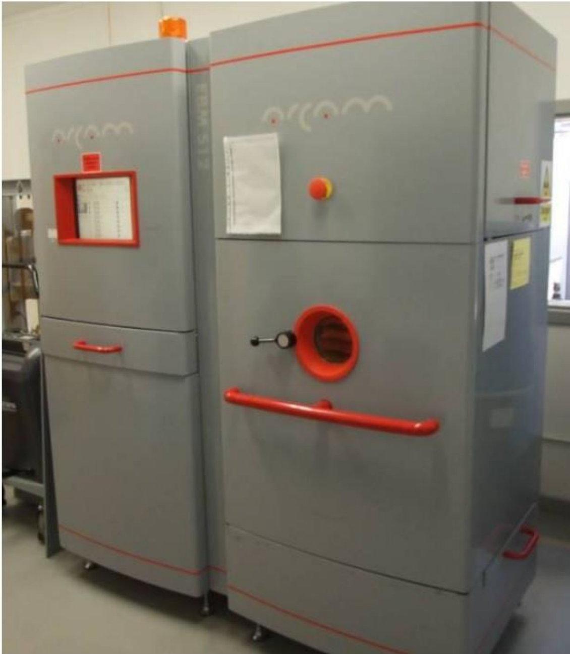
Figure 3.5 Photograph of the Arcam S12 EBM machine; the left side contains the work chamber while the right side contains the machine control unit
