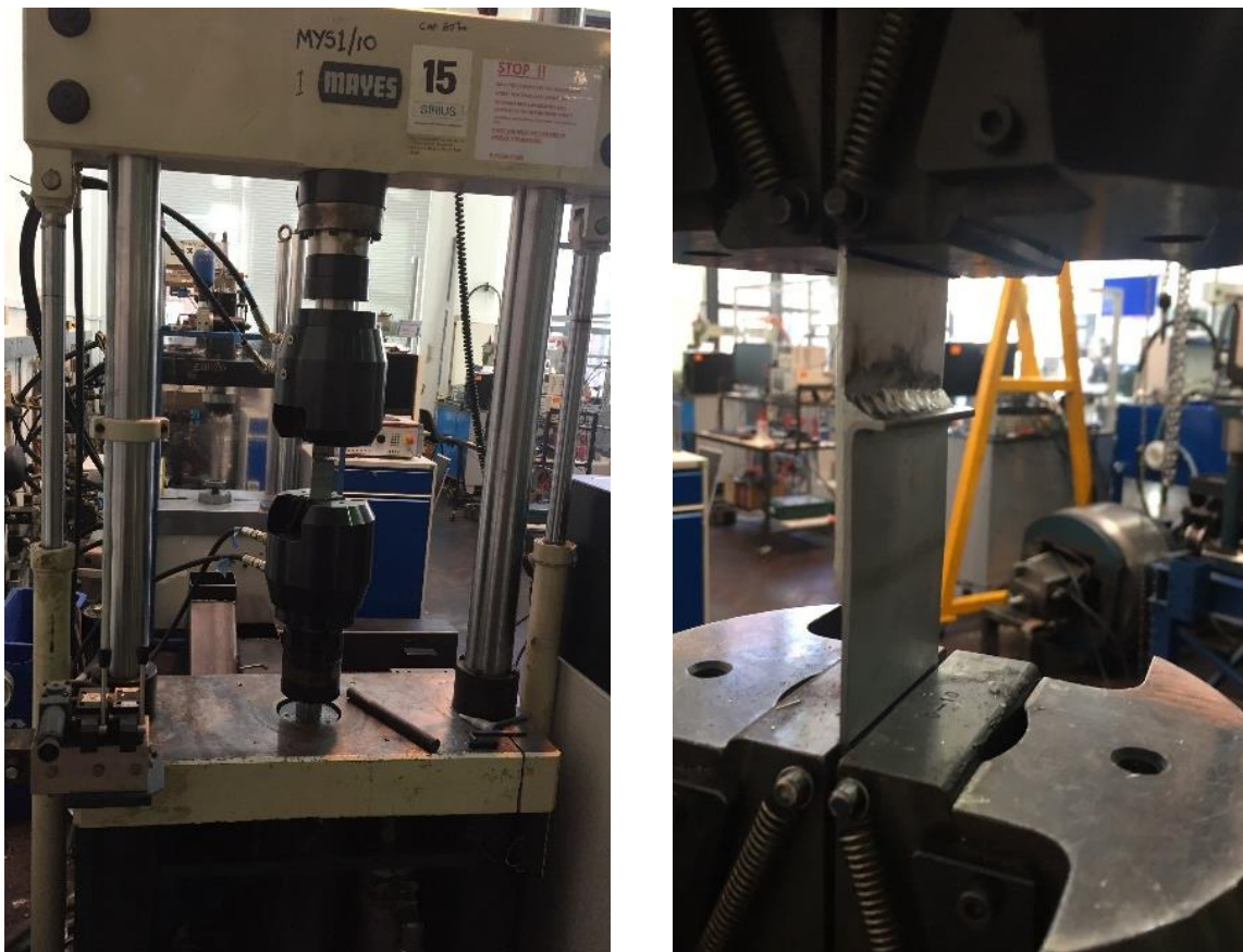
(a) (b) Figure 5.6 MAYSE uniaxial fatigue machine (a), hydraulic grips (b).
