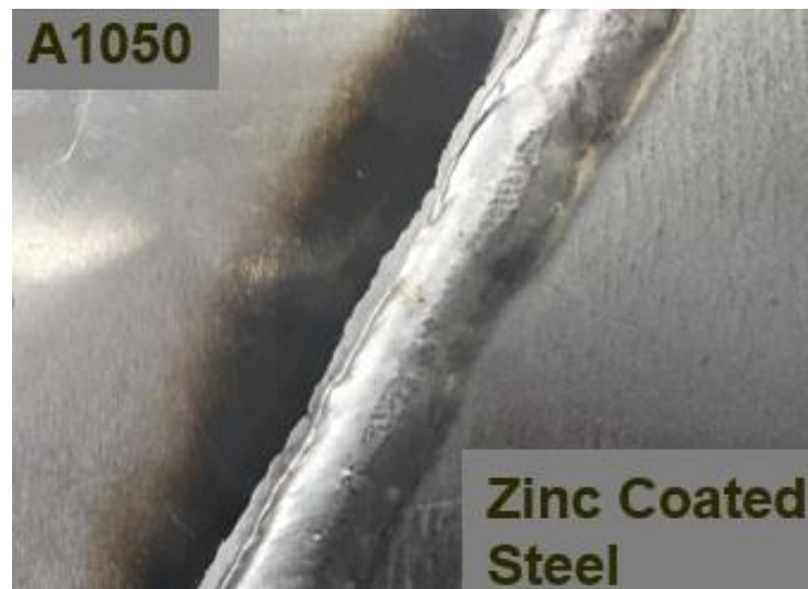
Figure 2.7 Spatter-free welding achieved by using EWM coldArc welding technology.
