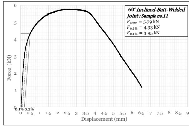
Figure C.6 Force vs. displacement curve for 60° inclined butt-welded joints (short term) (continue)
