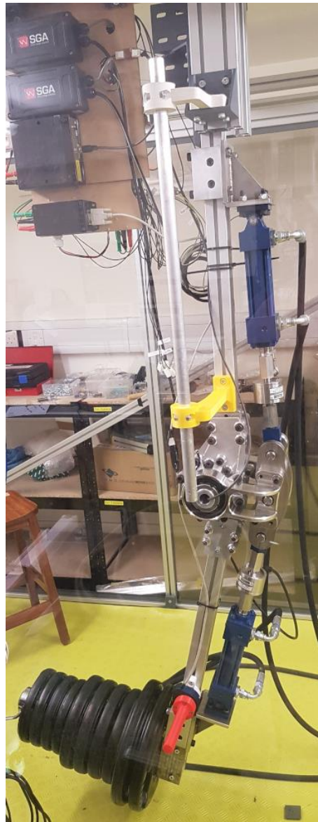
Figure K.1: Complete single joint test rig for the University of Leeds enhanced exoskeleton [K.1]
