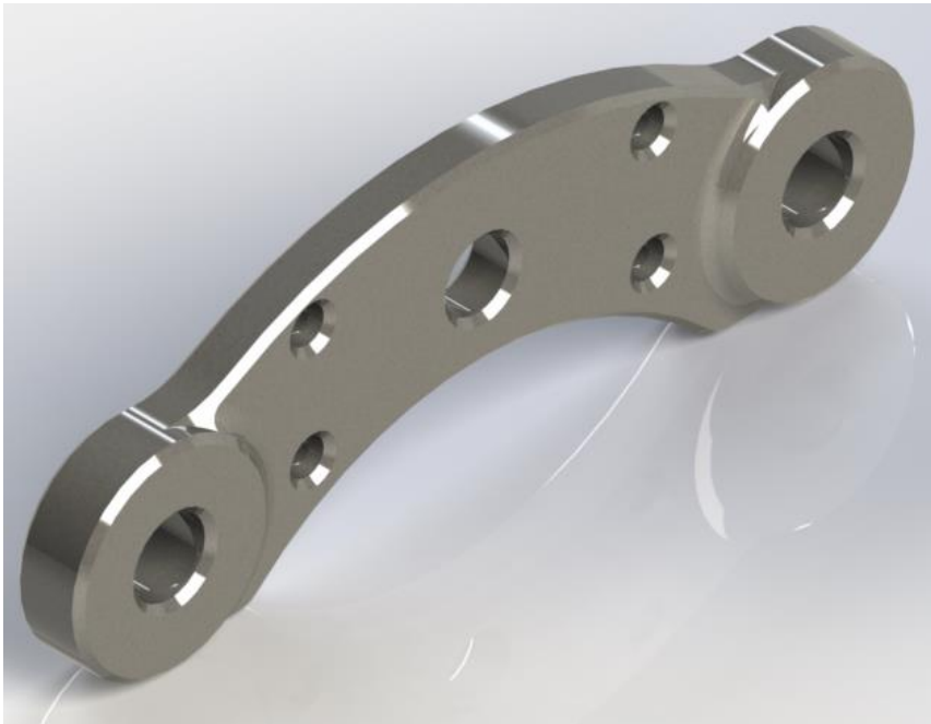
Figure H.1: Horizontal transfer plate
