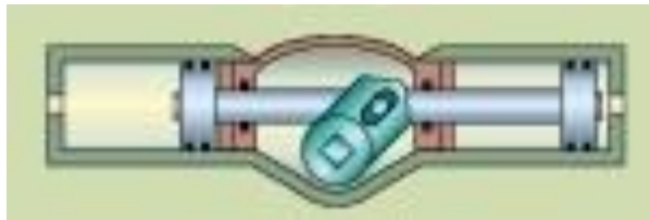
Figure 2.14: Scotch yoke actuator overview [35]
