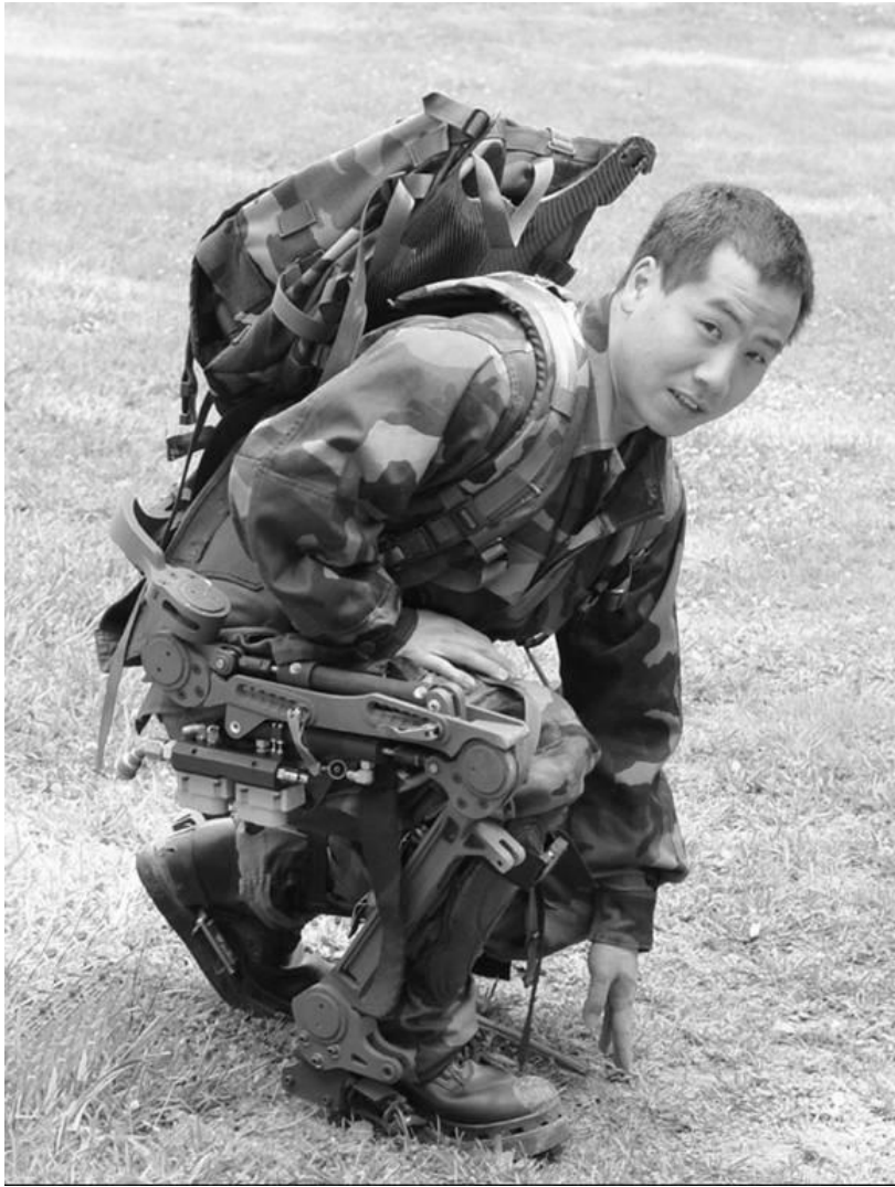
Figure G.1: Mock-up design for the BLEEX system showing squat motion [G.1]
