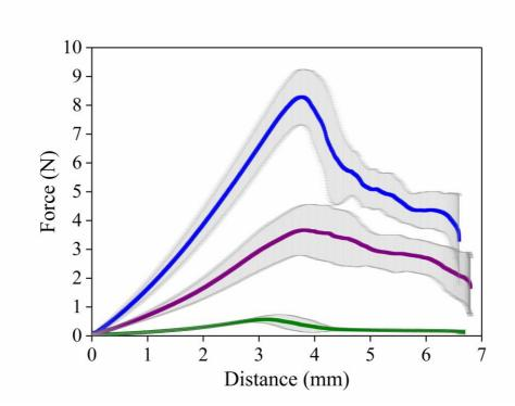
Figure 5.1. Mean ( $\pm$  SD) force over distance curve of the hydrogels obtained from puncture tests with a Volodkevitch probe (first bite), with  $3\kappa C$  ( $\blacktriangle$ ), 1.5 $\kappa$ C0.5NaA ( $\blacklozenge$ ) and 2.4 $\kappa$ C0.2CaA<sub>300</sub> ( $\bigcirc$ ).
