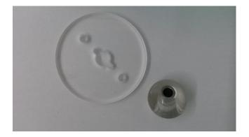
Figure 1.7. Commercial PDMS ball and disc tribology specimens.
