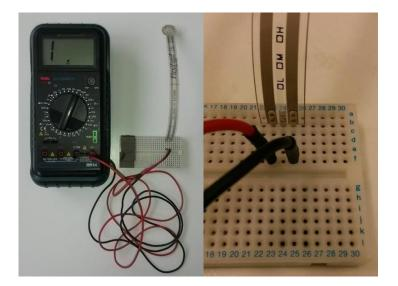
Figure 1.11. Multi-meter and flexisensor with silicon disc for bite force measurements, connected through a bread board.
