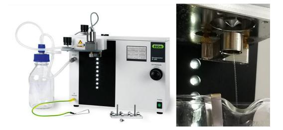
Figure 3.5. Buchi Encapsulator<sup>®</sup> set-up (left) and dropping mechanism of the NaA solution into a water bath with Ca<sup>2+</sup> ions (right).
