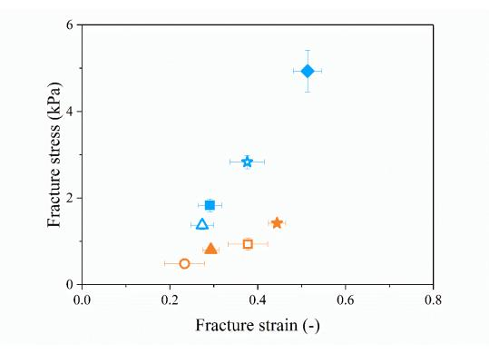
Figure 3.8. Mean ( $\pm$  SD) fracture stress and fracture strain curve of puncture tests with Volodkevitch probe of mixed  $\kappa$ C and NaA hydrogels, with concentrations  $1\kappa$ C1NaA ( $\bigcirc$ ),  $1.4\kappa$ C0.6NaA ( $\blacktriangle$ ),  $1.5\kappa$ C0.5NaA ( $\Box$ ),  $1.8\kappa$ C0.2NaA ( $\star$ ),  $1.5\kappa$ C1.5NaA ( $\triangle$ ),  $1.8\kappa$ C1.2NaA ( $\blacksquare$ ),  $2.25\kappa$ C0.75NaA ( $\star$ ) and  $2.7\kappa$ C0.3NaA ( $\blacklozenge$ ).
