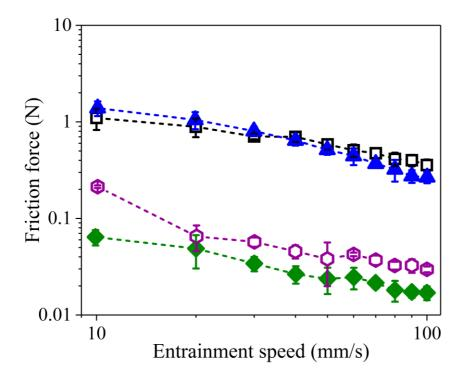
Figure 5.2. Mean friction force ( $\pm$  SD) of  $3\kappa$ C ( $\triangle$ ), 1.5 $\kappa$ C0.5NaA ( $\blacklozenge$ ) and 2.4 $\kappa$ C0.2CaA<sub>300</sub> ( $\bigcirc$ ) gel bolus filtrates, after simulated oral processing with artificial saliva ( $\Box$ ), at 37 °C as a function of entrainment speed in the mixed lubrication regime.
