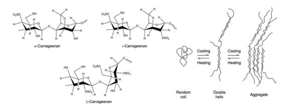
Figure 3.1. Schematic representation of the molecular structures of  $\kappa$ -, *i*- and  $\lambda$ -carrageenan (left), and gelation mechanism (right), adapted from Kariduraganavar, Kittur and Kamble (2014) and Williams and Phillips (2003).
