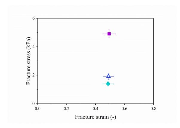
Figure 3.9. Mean ( $\pm$  SD) fracture stress and fracture strain curve of puncture tests with Volodkevitch probe of mixed  $\kappa$ C hydrogels of various concentrations and an added layer of CaA beads, with 1.6 $\kappa$ C0.2CaA<sub>300</sub> ( $\bullet$ ), 1.6 $\kappa$ C0.2CaA<sub>1000</sub> ( $\Delta$ ), 2.4 $\kappa$ C0.2CaA<sub>300</sub> ( $\bullet$ ).
