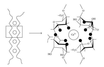
Figure 3.4. Schematic illustration of the "egg-box model" gel structure for alginates in presence of calcium ions (Braccini and Pérez 2001).
