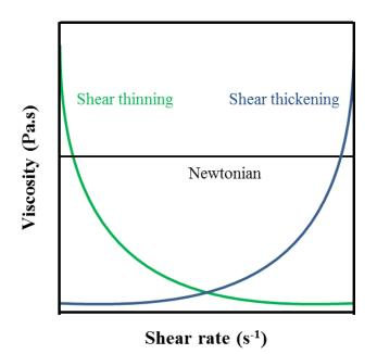
Figure 1.4. Typical flow-curves for Newtonian and non-Newtonian fluids (van Vliet 2014).
