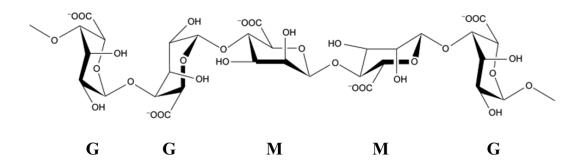
Figure 3.3. Schematic representation of the molecular structure of alginate, as adapted from Draget (2000) and Kariduraganavar, Kittur and Kamble (2014).
