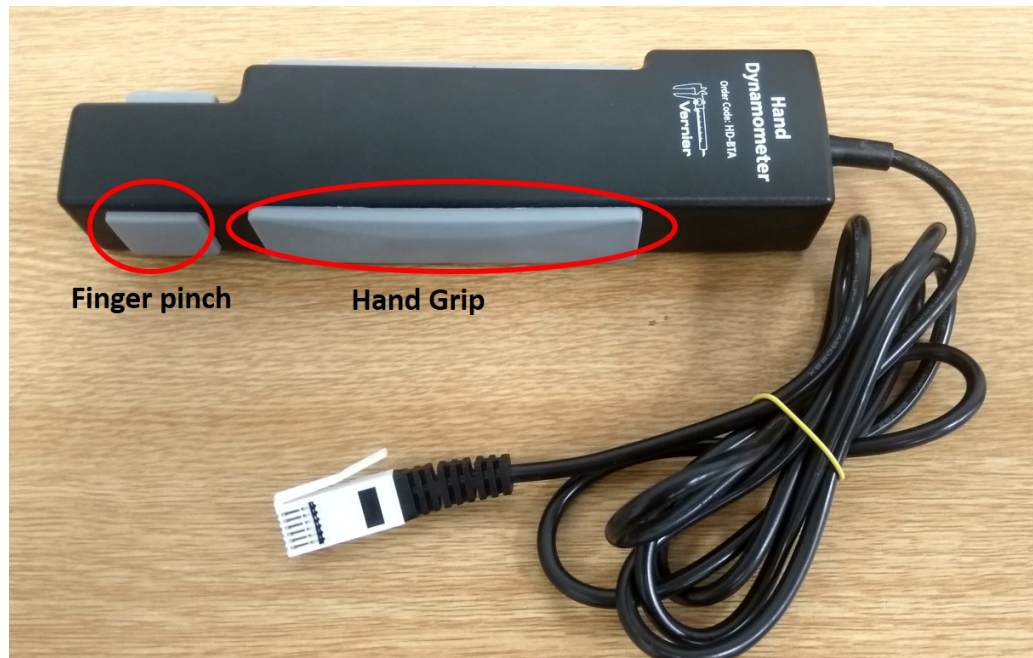
Figure 3.8: The hand dynamometer that has been used to measure force exertion from the subject. This sensor uses the analogue port as its input. Unique design for a separate task can be seen in the figure, as highlighted in the red circles. The small circle represents the force sensor location for the finger pinch and the bigger circle designed for hand grip force.
