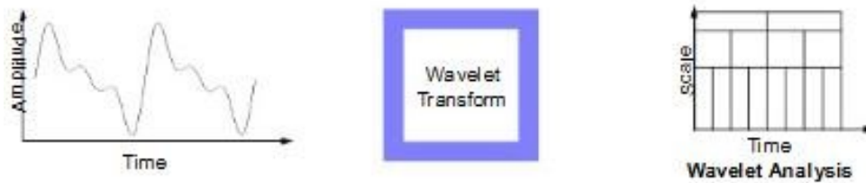
Figure 4.5: The general approach of Wavelet transform process.
