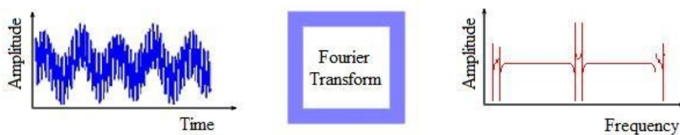
Figure 4.2: The Fourier transform (FT) is the general practice in the measurement of time series signal. The fundamental practice of FT is changing domain of operation in the TD into the FD. (Adapted from Matlab software application)
