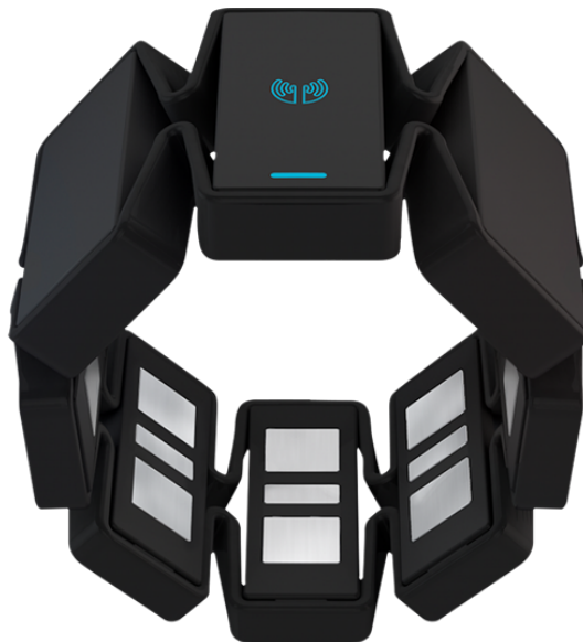
Figure 2.3: The Myo Armband, a low-cost commercial sEMG device [78].
