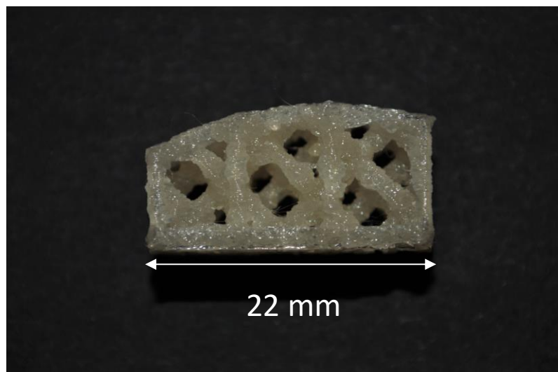
Figure 5.26. Detail photograph of framed 3D-mesh prototype produced on VB-PLA through the procedure described in this section. Lateral view.
