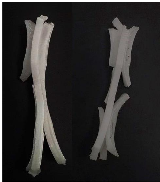
Figure 5.13. Detail photograph of VB-PLA 63 mm-long tensile specimens at 24h (left) and 48h (right) after mADT. Depictions of lateral views. The dismantling period for this material under mADT conditions is considered to be 24 hours, since the specimens become far too distorted for mechanical testing. Lower time periods displayed no significant changes.
