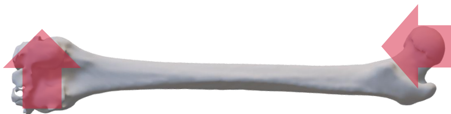
Figure 5.4. Laser scanned model femur, proximal to distal sweep over the femur head and lateral to medial sweep of the posterior femur condyles.
