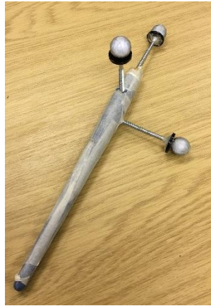
Figure B1. Paint brush wand design with three retro-reflective markers implemented and masking tape applied to minimise unwanted reflection.
