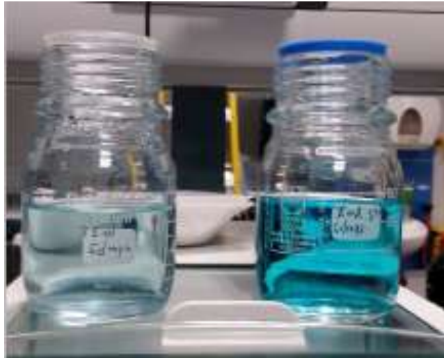
Figure 3.5. Dissolved hydrogen experiment with MB-Pt reagent; the right bottle is the reagent in distilled water and the left is the reagent after bubbling with the H 2 /N 2 gas mixture.
