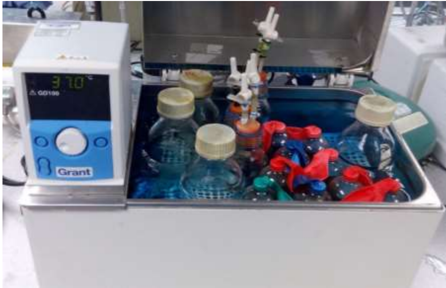
Figure 3.6. BMP trial experiments with hydrogen injection for test of reactor suitability.
