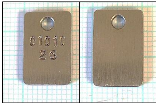
Figure 10 Back and front of AISI C1010 coupons. Dimensions: L: 14 mm, W: 9 mm. Mounting hole diameter: 3 mm, and thickness: 1 mm.
