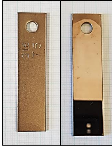
Figure 31 Left: Unpolished, rough surface on the back side of the coupon compared to (right) mirror-polished front side, reflecting surroundings as the photo was taken.
