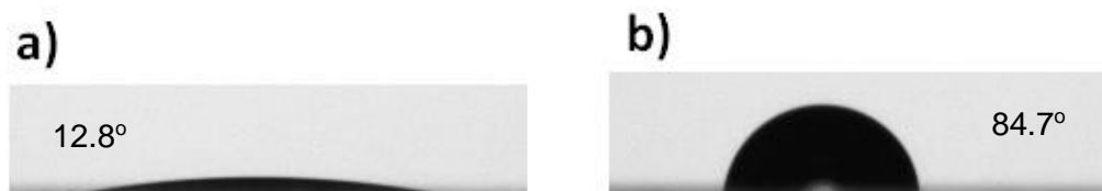
Figure 5.5 The contact angle of (a) untreated ZnO thin film and (b) HMDS-ZnO.
