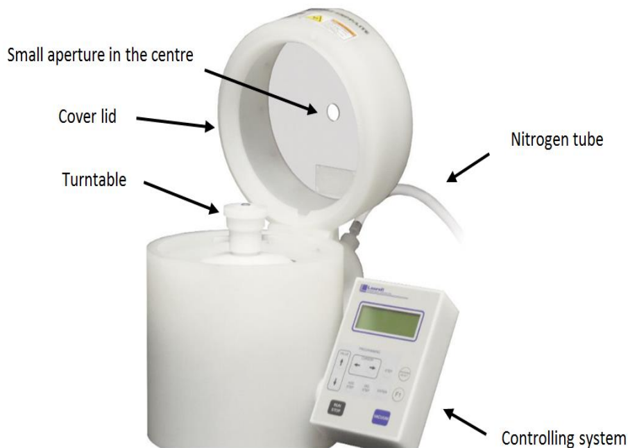
Figure 4.6 Spin-coater used in our laboratory (WS-400BZ-6NPP/LITE Model).
