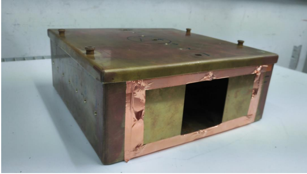
Figure 5. 3. Photograph of the 300mm×300mm×120mm enclosure under test with the 75mm×75mm square aperture.
