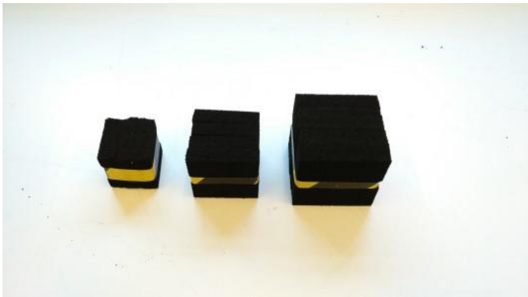
Figure 5. 8. Photograph of the absorbing cubes used in this thesis. Their side lengths are (from left to right) 55mm, 70mm and 90mm.
