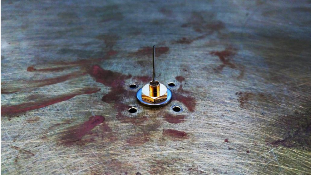
Figure 5. 24. Close up look at the monopole, which is antenna 3 shown in figures 5.22 and 5.23.
