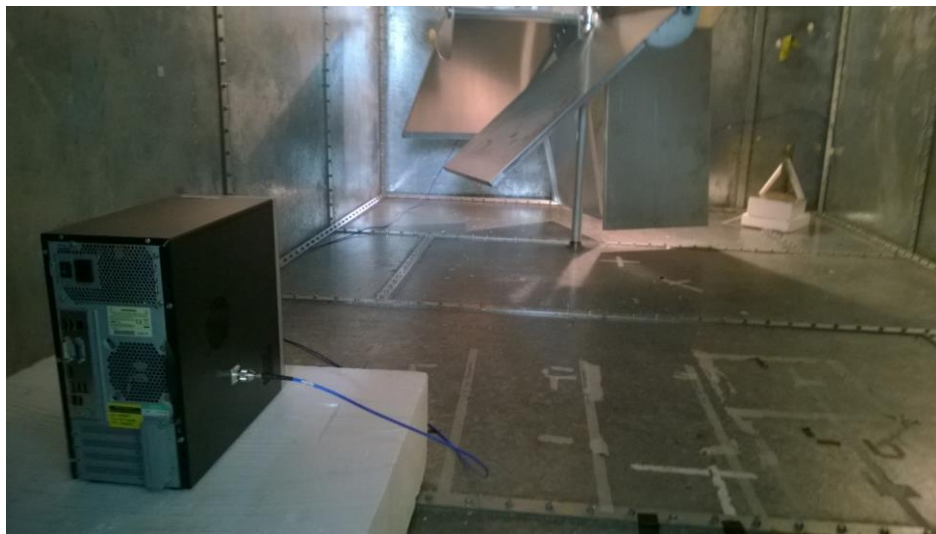
Figure 4. 2. Photo of the shielding effectiveness measurement configuration with the presence of the computer enclosure.
