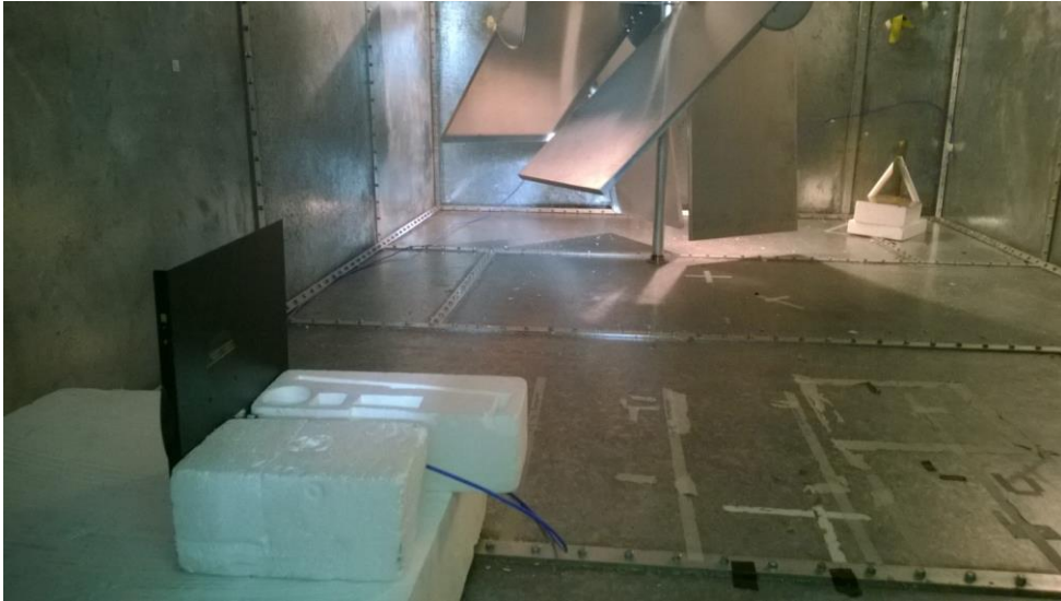
Figure 4. 3. Photo of the shielding effectiveness measurement configuration with the absence of the computer enclosure.
