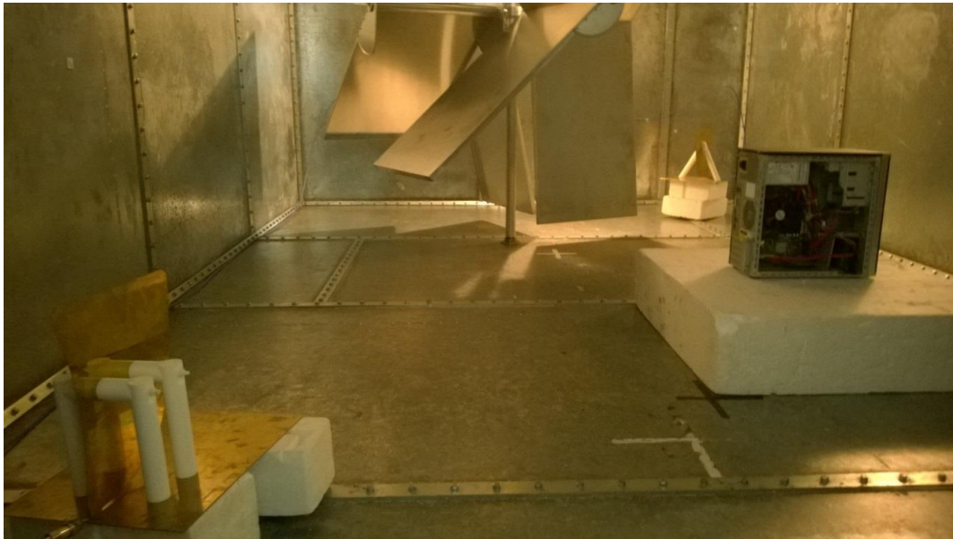
Figure 4. 27. Photograph of the Absorption cross section measurement configuration of the computer at position 1 in the reverberation chamber at the University of York.
