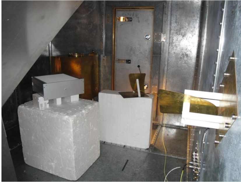
Figure 4. 7. Photo of the shielding effectiveness measurement configuration in the reverberation chamber at the University of York.
