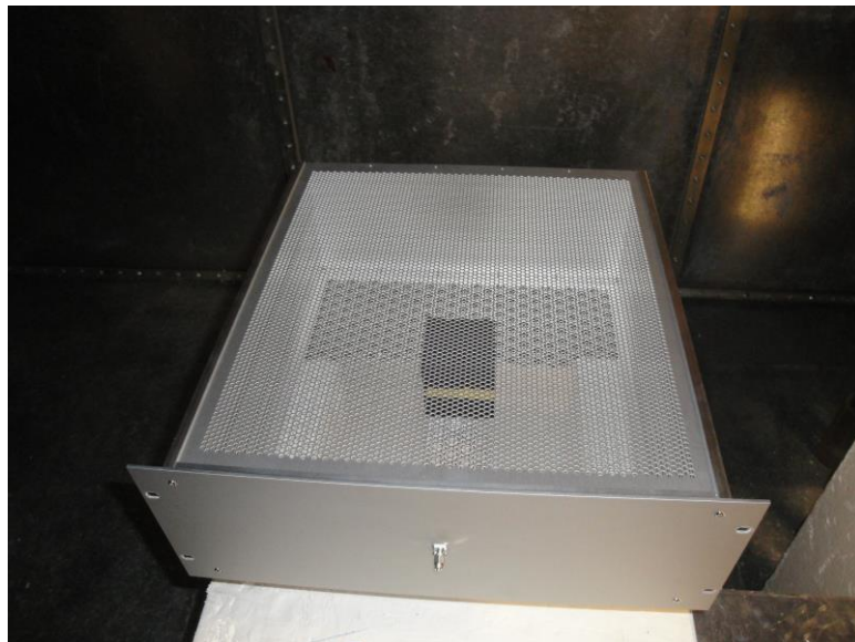
Figure 4. 6. Photo of the top view of the enclosure, showing the absorbing cube inside it.
