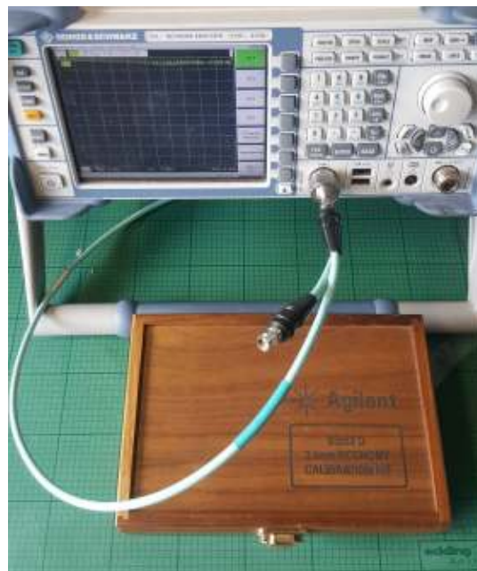
Fig. 3.1 A capture of the Vector Network Analyser with a coaxial connected to Port 1
