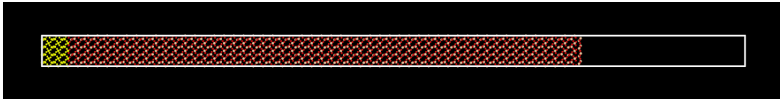
Figure 6.1: The initial system set-up for the LAMMPS NEMD BKS shock. The flyer-plate is in yellow and launched with its initial velocity and feels no response force. Note the addition of a vacuum gap compared to Lennard-Jones simulations to reduce interaction along the direction of the shock.
