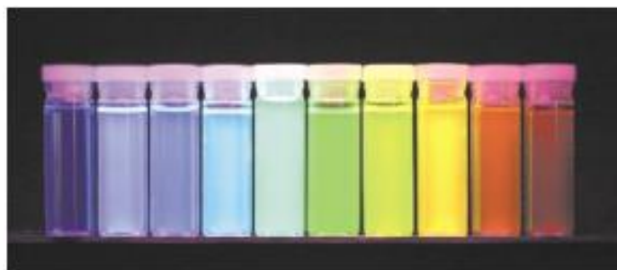
Figure 1.1.3: Ten easily distinguishable emission colours of (CdSe)ZnS quantum dots ranging from blue to red, with emissions located at 443, 473, 481, 500, 518, 543, 565, 587, 610 and 655 nm respectively excited by a single light source. Reprinted from reference. 10
