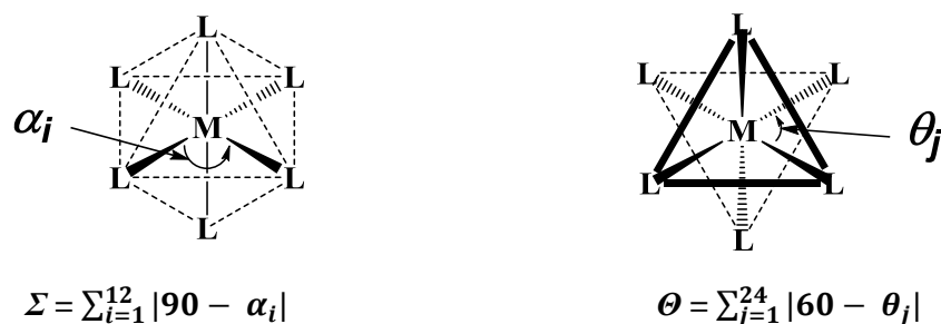
Figure 1.15: Where \alpha_i are the 12 cis N-Fe-N angles and \theta_j are 24 unique N-Fe-N angles measured from the triangular projections along the pseudo-threefold axis. Both \Sigma and \Theta are usually much larger for HS state than the LS.
