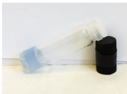
Figure 3.17: Picture of the Ni[2]B-AgBF 4 CPG after 20 months.
