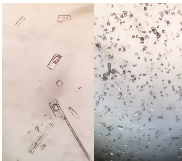
Figure 3.25: Photography taken from the optical microscope of the crystals before (left) and after (right) the self-recrystallization.
