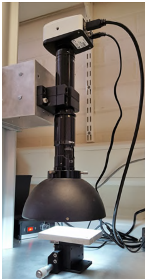
Figure 3-19. Experimental set-up of Luminera Infinity 3 camera with a Navitar 12X zoom lens and diffuse lighting.
