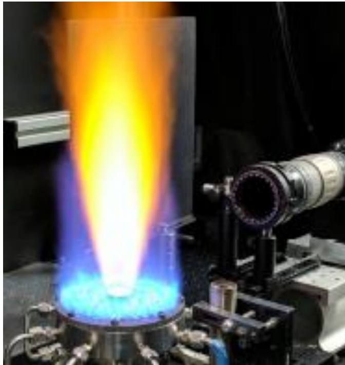
Figure 5.5 Hi-pilot Michigan burner by (Driscoll et al., 2017).
