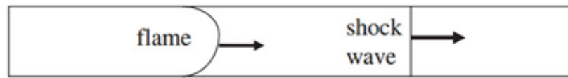
Figure 4.1 Flame and shockwave propagation in an open-ended tube. Ignition initiated from the closed end (Bradley et al., 2008).
