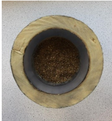
Figure 3.13: Top view of the conductivity cell body showing the external insulation
