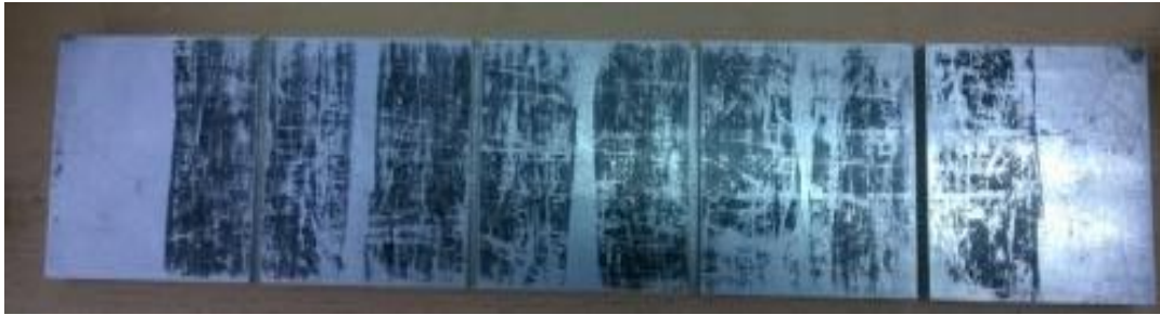
Figure 7.12: Crack depth samples. Slits of different depths cut into the metal is used to mimic the effect of a crack at different depths
