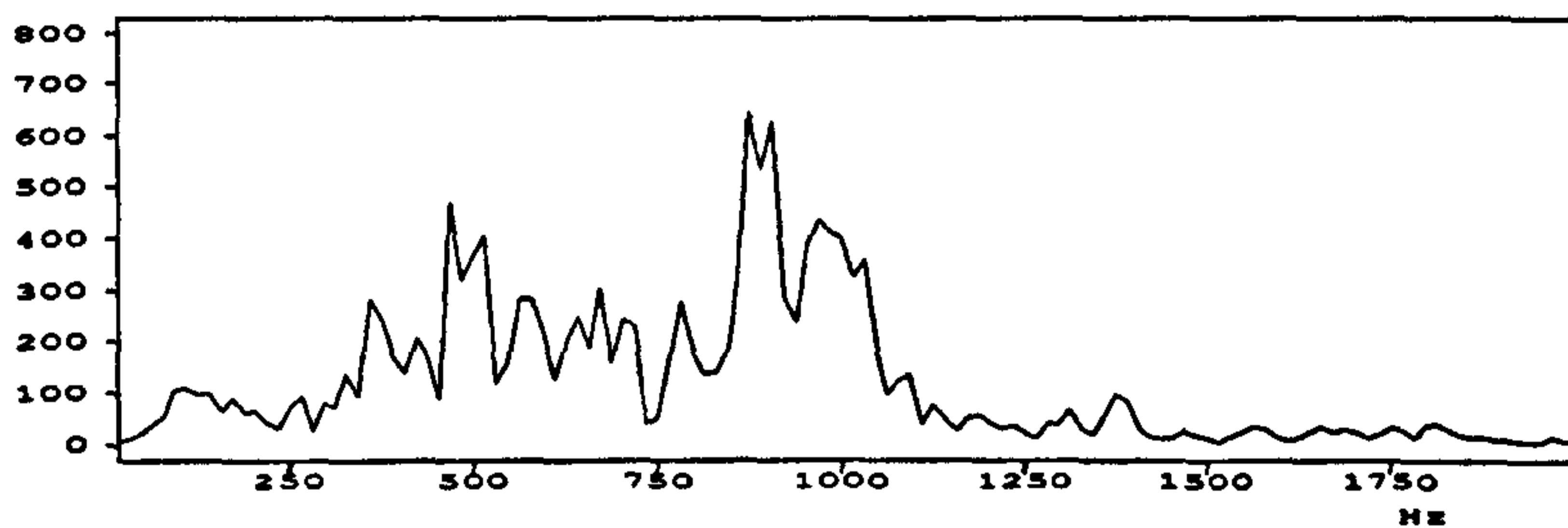
FIGURE 8.13 Frequency domain spectra for hammer shot traces in figure 8.12
