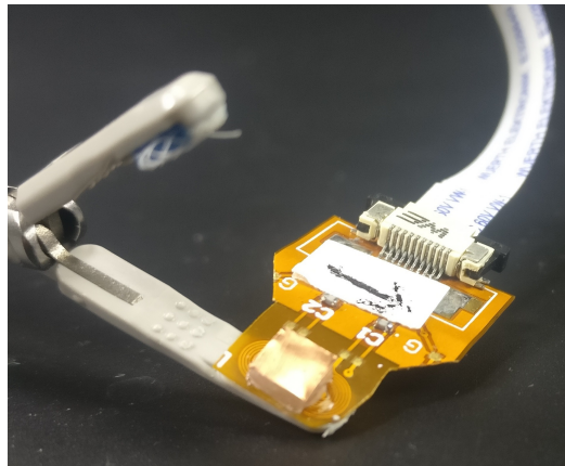
Fig. 7.9 (a) Schematic of the miniaturised coil, indicating coil and target sizes; and (b) The manufactured prototype, with the sensor mounted on a toothless 5 mm laparoscopic grasper (Epix, Applied Medical)
