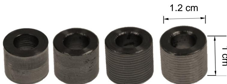
Figure 3-7 Images of the RCE samples with different surface roughnesses.
