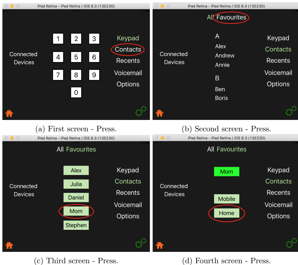
Figure 3.7: Medium HMI task. The home screen is illustrated on top and the succession is from left to right, top to bottom, as denoted by the captions. Red circles denote the areas on the screen (virtual buttons) that the user needed to press in order to move to the next screen and complete the task.
