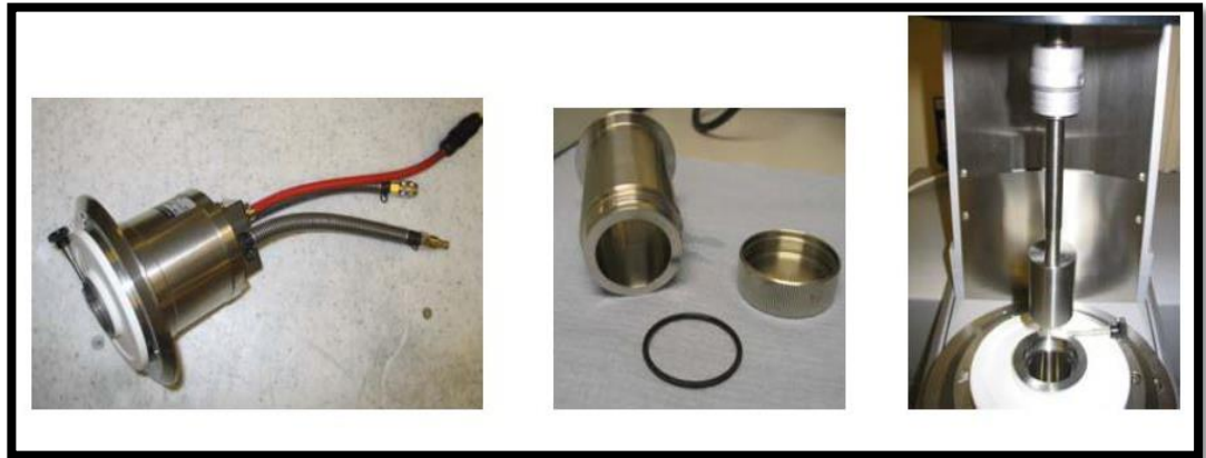
Figure 3-9 Viscosity measuring cell; Bob and cylindrical cup [103].
