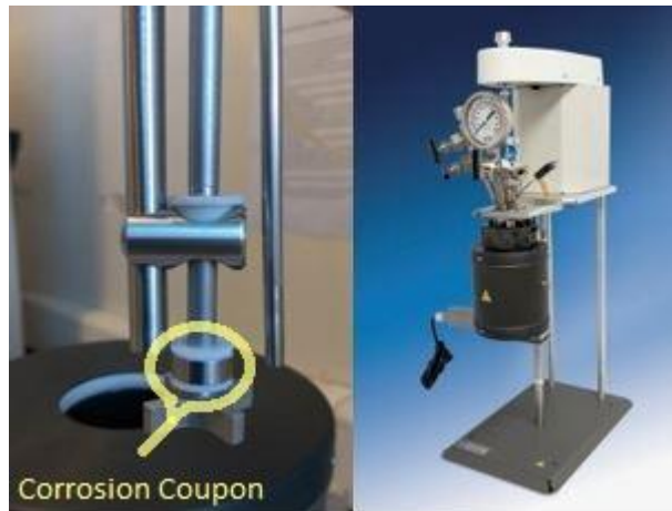
Figure 3-17 Erosion-corrosion experiment set up
