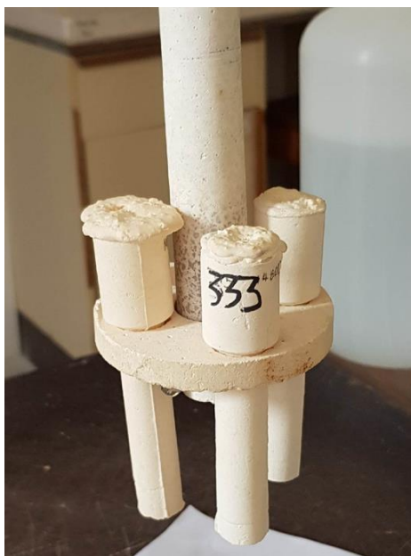
Figure 4-8: dumbbell shaped finger samples for dynamic corrosion on a sample holder.
