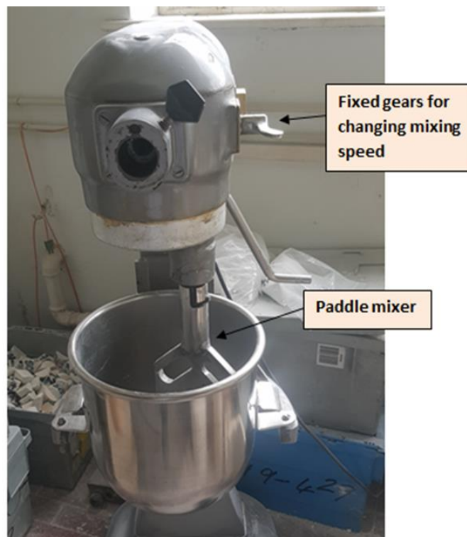
Figure 4-2: Hobart Mixer used to mix 5-10kg batches of the developed mix formulations at PSR-ltd. Picture courtesy of PSR-Ltd.
