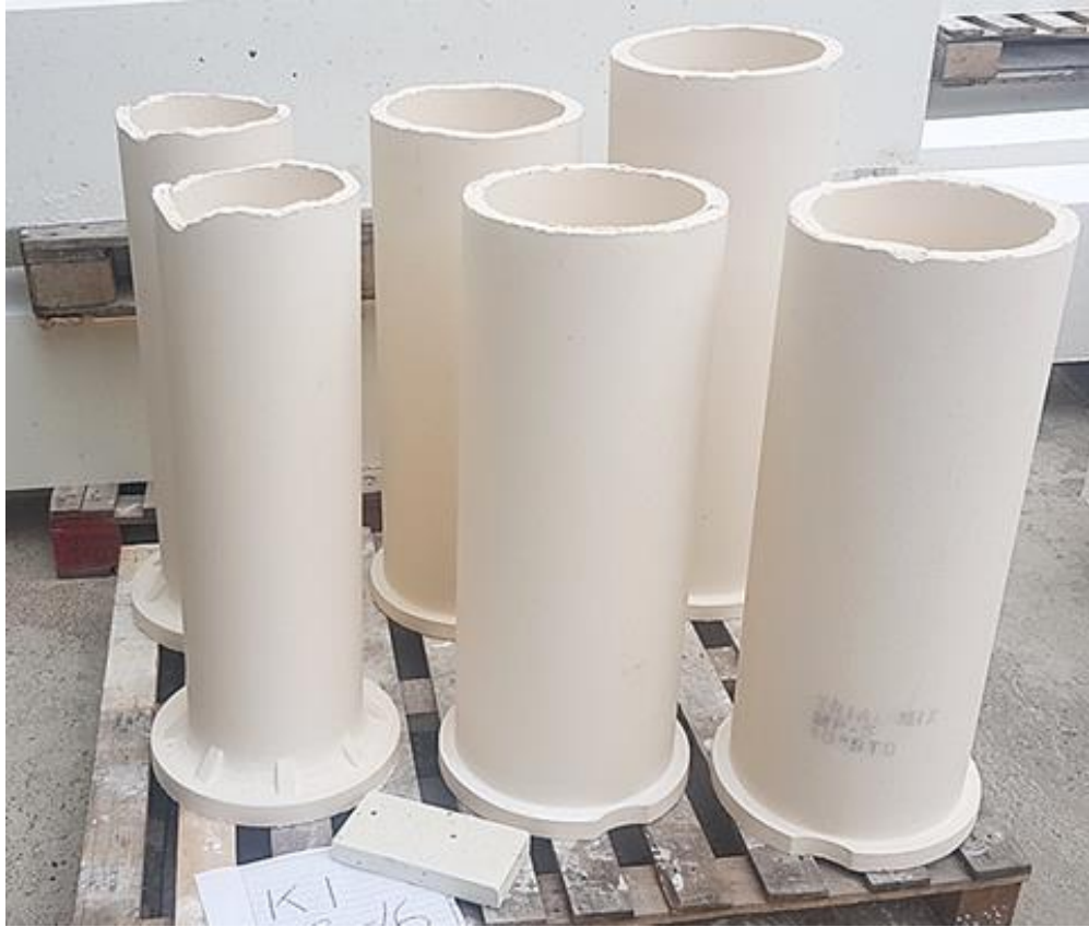
Figure 5-18: Feeder tubes cast from AZS-01 factory-scale mix.
