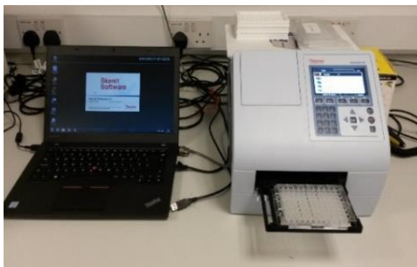
Figure 16: Thermo Scientific MultiSkan GO! Spectrophotometer. Optical densities for each ELISA assay were quantified using the spectrophotometer at the end of each experiment. Results were exported and used for calculating calibration curves and determining sample concentrations.
