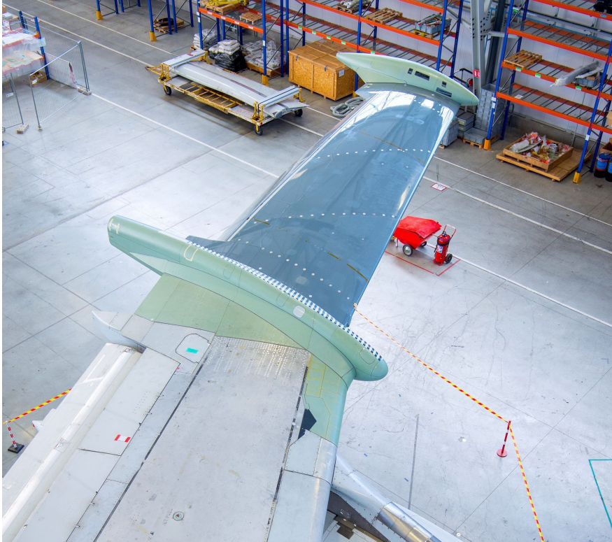
Figure 1.2: Airbus BLADE NLF wing section (Photo: P. Pigeyre / Master Films. Copyright: Airbus) [16].
