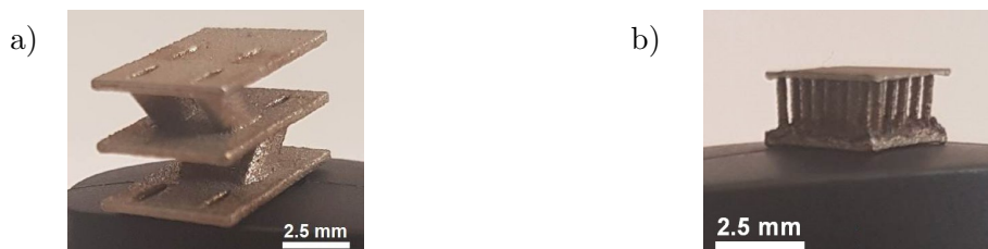
Figure 6.11: Scaled down versions of: a) Inter-layer and b) Cylindrical fins manufactured using the SLM process.
