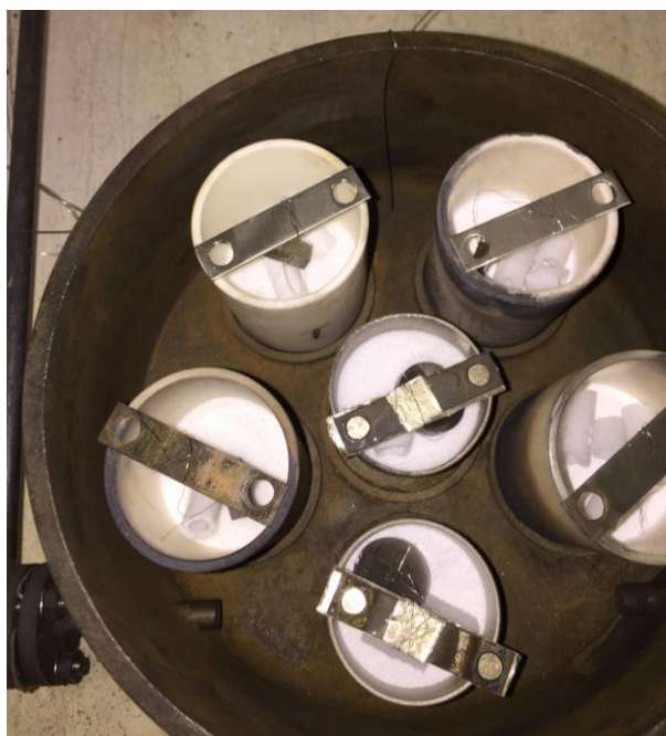
Figure 23 – Samples suspended by nickel wire in as-received salts.
