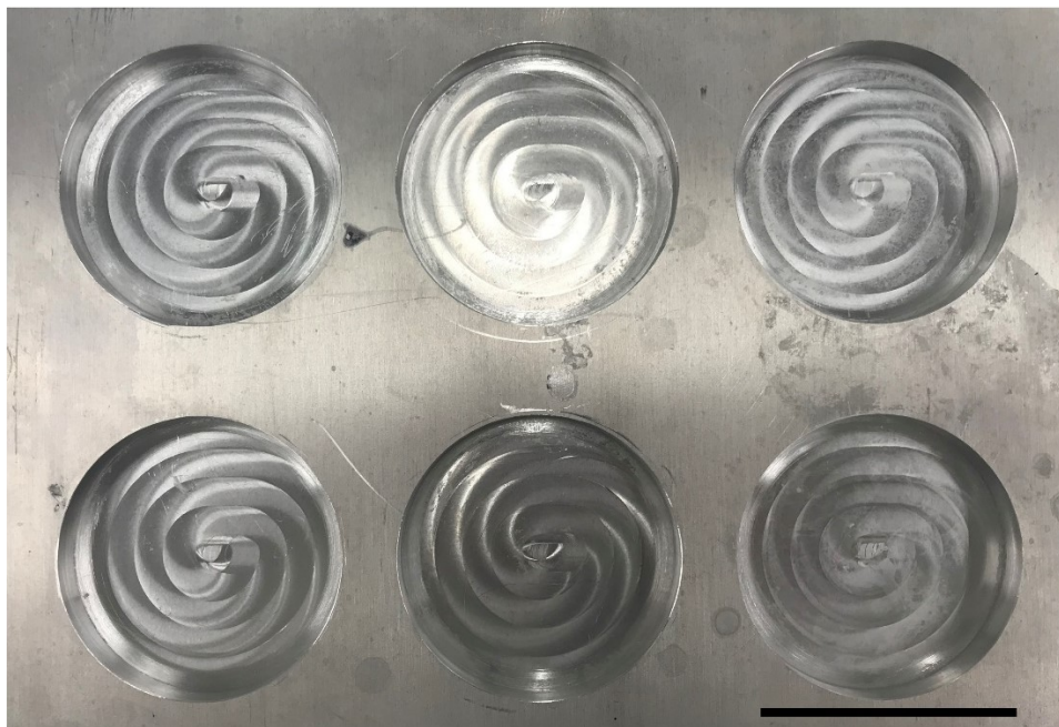
Figure 3.1. Aluminium tray mould with 6 wells for random orientation (mould-random) scaffold fabrication. Scale bar is 5 cm.
