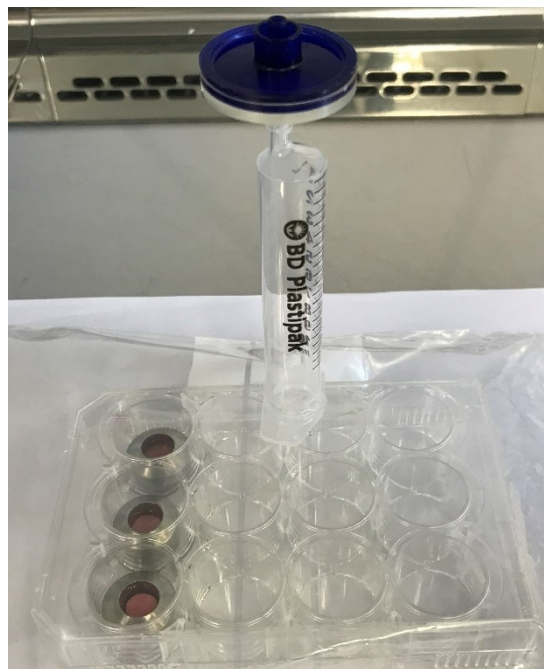
Figure 4.3: Image showing the PGSU-BM ready for dynamic seeding. The scaffolds are fixed in a surgical stainless-steel ring and overlaid with cell/media suspension. The well-plate was then placed in a sterile plastic bag with a syringe and a syringe filter to sterilise the returning air while ventilating.
