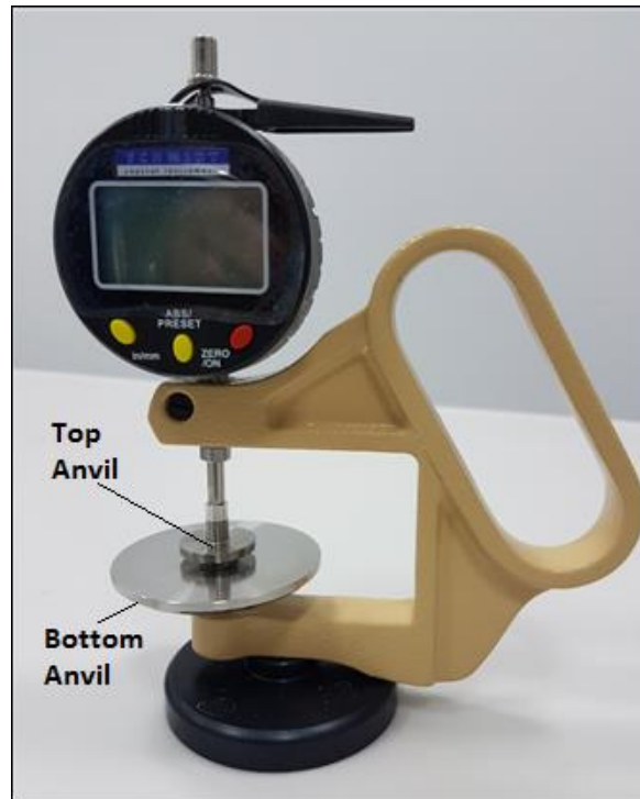
Figure 2.25 Digital Thickness Gauge J-40 V (James H. Heal and Company Limited)
