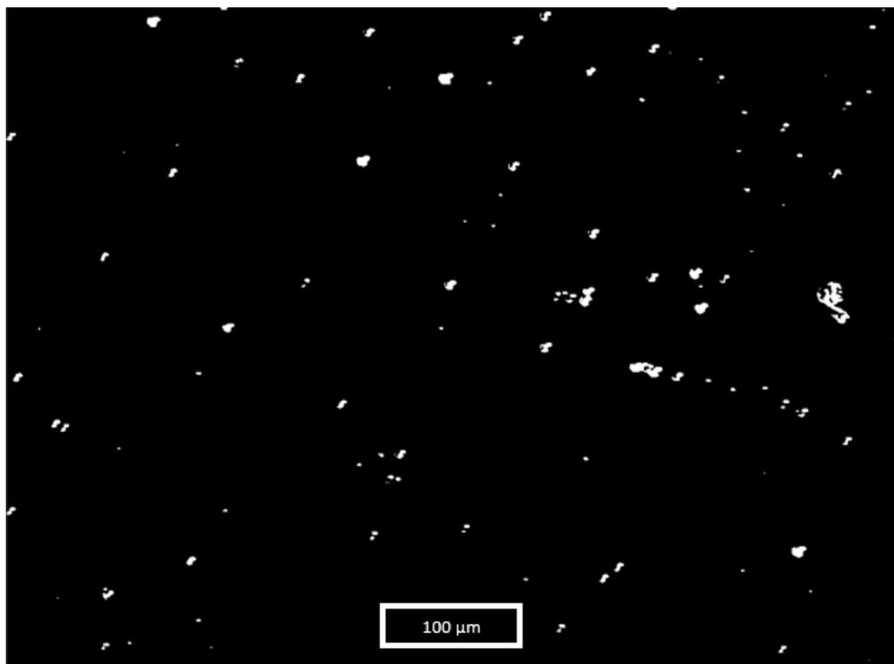
FIGURE 5.11: Nomarski image of G120 segmented using Otsu's method, showing the droplet-like defects as white features against a black background
