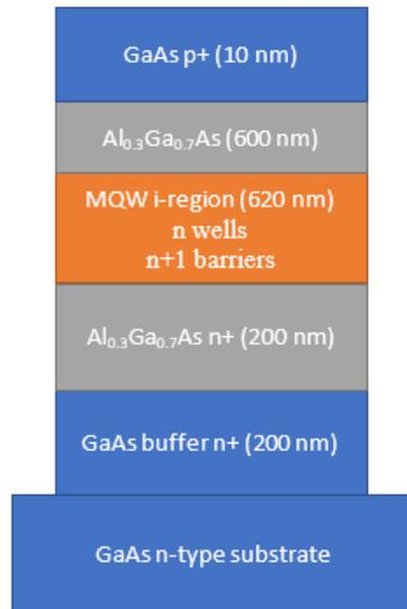
FIGURE 5.1: Nominal growth structure of series C GaAsBi/GaAs MQWs grown by Richards et al. For the structure of the i-region, see table 5.1
