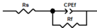
Figure 6.12 Equivalent circuit corresponding to the EIS spectra of uncoated stainless steel after exposure to 3.5%NaCl
