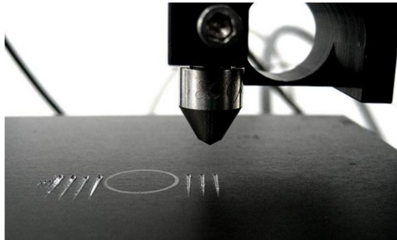
Figure 4.8 Image of the tip over the scratches of a tested sample [201]
