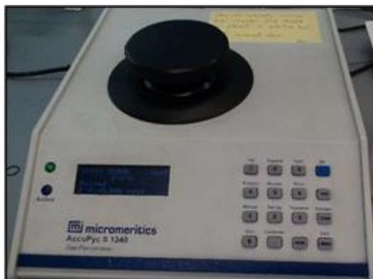
**Figure 3.6. Images of AccuPyc II 1340 Automatic Gas Pycnometer**
