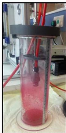
**Figure 6.5. Set-up for spray rate measurement**
