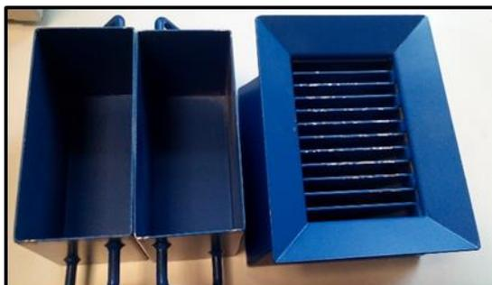
**Figure 4.2. A riffle sample splitter used for sampling**
