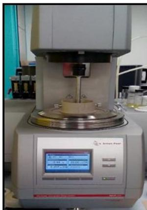
**Figure 3.8. MCR 502 Anton Paar Rheometer**
