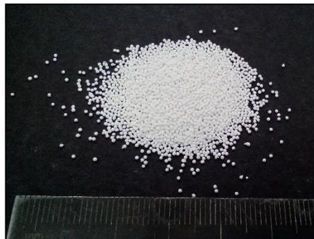
**Figure B2: Uncoated Zirblast particles**
