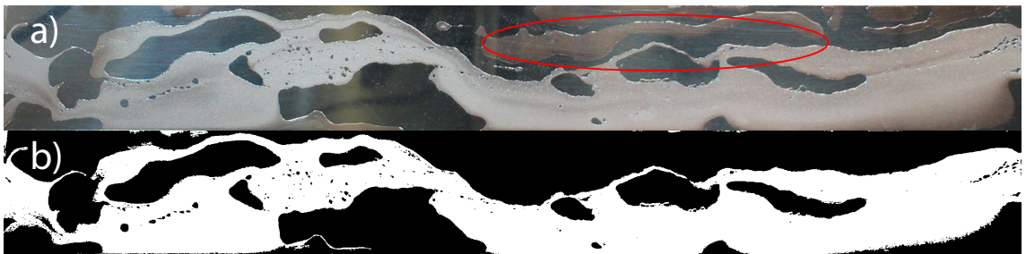
Figure 5.13: Example of threshold achieved with final lighting set-up. a) shows an unedited image of the coalescer and b) the final threshold.
