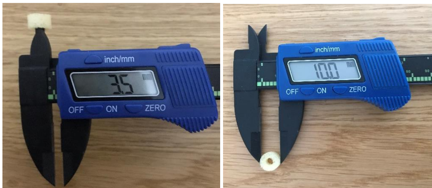
Figure 3.4 Epilog Mini laser cutter machine (B) PU scaffold with initial size dimensions (C) Final size dimensions used for the in vitro 3D culture model.
