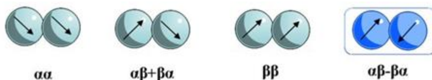
Figure 9: the four spin isomers of hydrogen. The three isomers in green are known as ortho -hydrogen, whereas the isomer in blue is known as para -hydrogen
