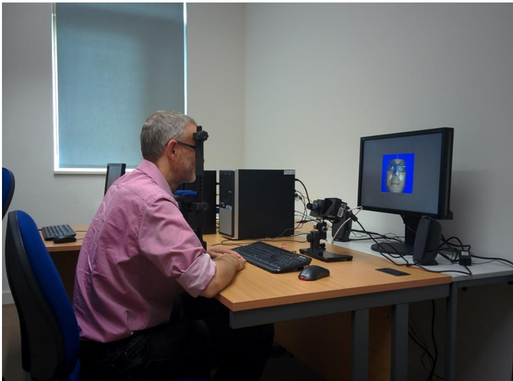
Figure 12 Eyelink eye tracker being used by a participant
