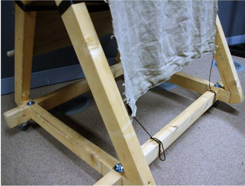
Figure 7.9: Tying down the loose side of the acoustic wind machine's cloth.
