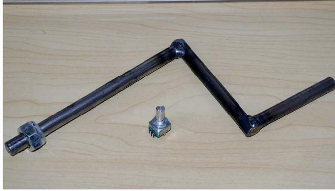
Figure 6.23: The first iteration of the digital crank handle and the digital rotary encoder it turned.
