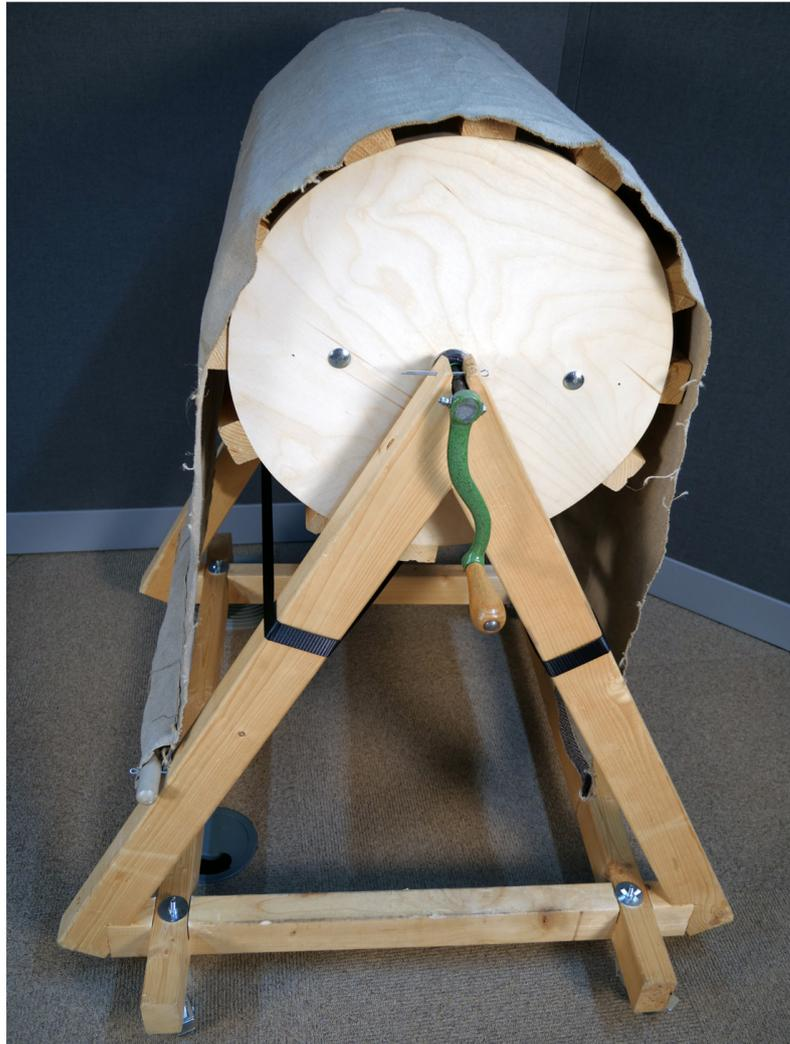
Figure 5.11: The completed acoustic wind machine with ratchet strap and wheels.
