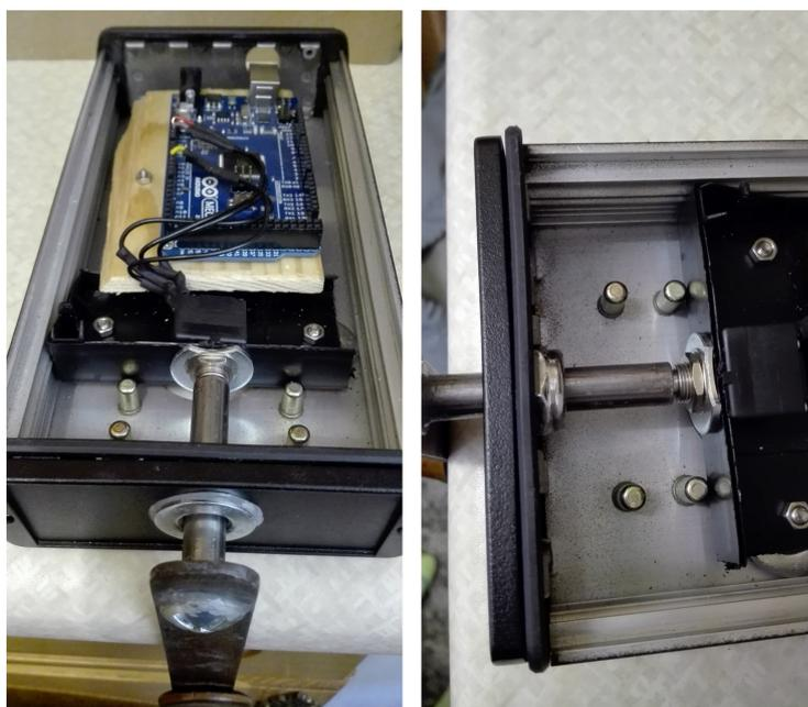
Figure 6.24: (L): The Arduino, rotary encoder and crank configuration in the metal enclosure. (R): Fixing the shaft of the crank handle to that of the rotary encoder.
