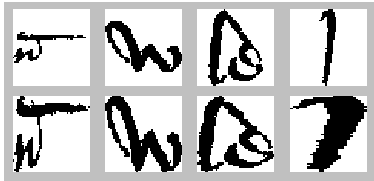
FIGURE 4.1: Comparison of graphemes produced by the ratio (top) and square (bottom) grapheme size normalisation methods
