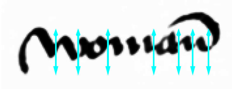
FIGURE 3.5: Example grapheme splitting points by the minima heuristic, as given in Bulacu and Schomaker (2007a)
