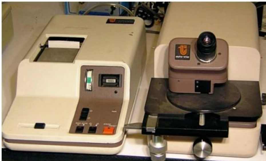
Figure3.6 Tencor alpha-step profiler
