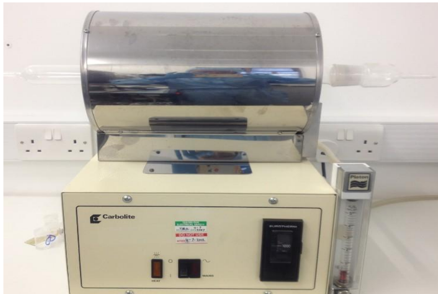
Figure3.1 Thermal Oxidation Furnace used for heat treatment
