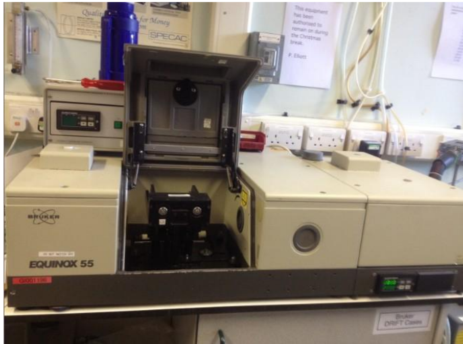
Figure 3.3 Equinox 55 Fourier Transform (FT-IR) spectroscopy
