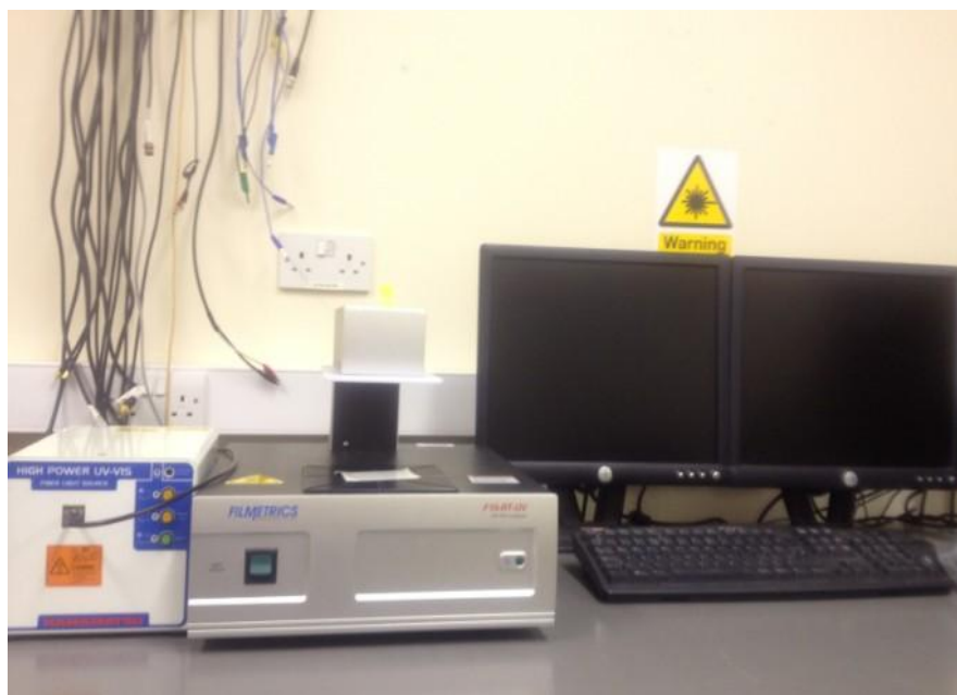
Figure3.2 Filmetrics F10-RT spectroscopy
