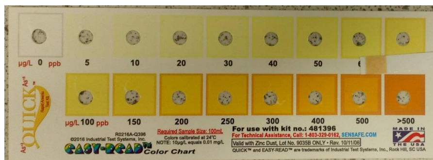
Figure 2.5.9 Shows the mercuric bromide paper colour after arsenic test kit on a solution that had a 2 mL hydrogel of DBS-CONH 2 (4.68 mM) and agarose (2.36 mg mL -1 ) placed in it for 72 hours
